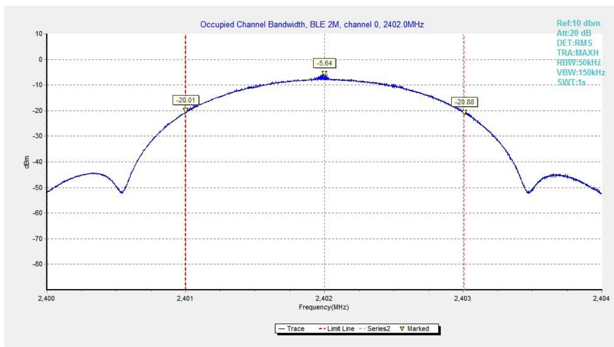
Fig.54 99% Occupied Bandwidth (Ch 0), LE 2M
