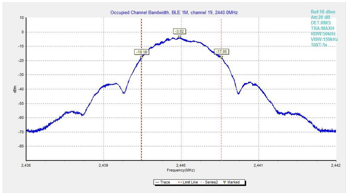
Fig.52 99% Occupied Bandwidth (Ch 19), LE 1M
