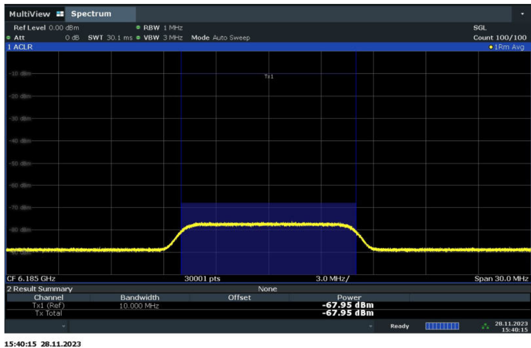
Fig.3 Contention Based Protocol 802.11ax-HE160 (ch6185MHz-middle-AWGN Signal Level)
