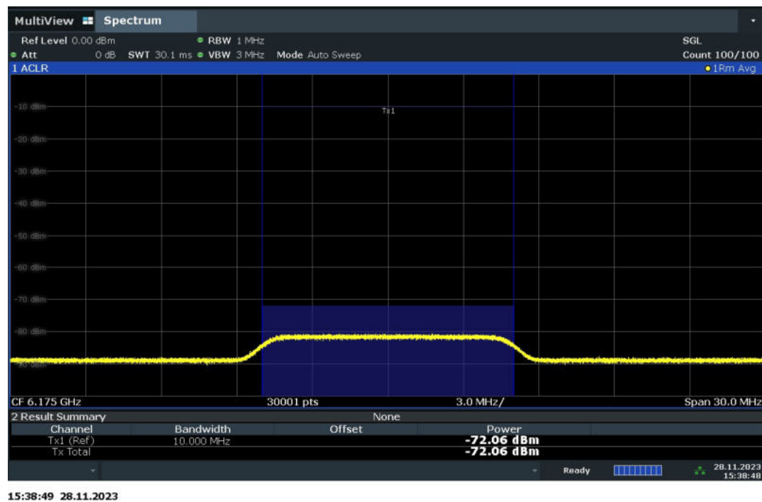
Fig.1 Contention Based Protocol 802.11ax-HE20(ch6175MHz-AWGN Signal Level)
