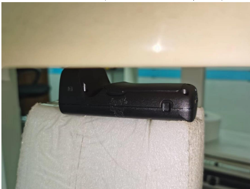
DUT without device holder (DUT direct contact with the phantom)
