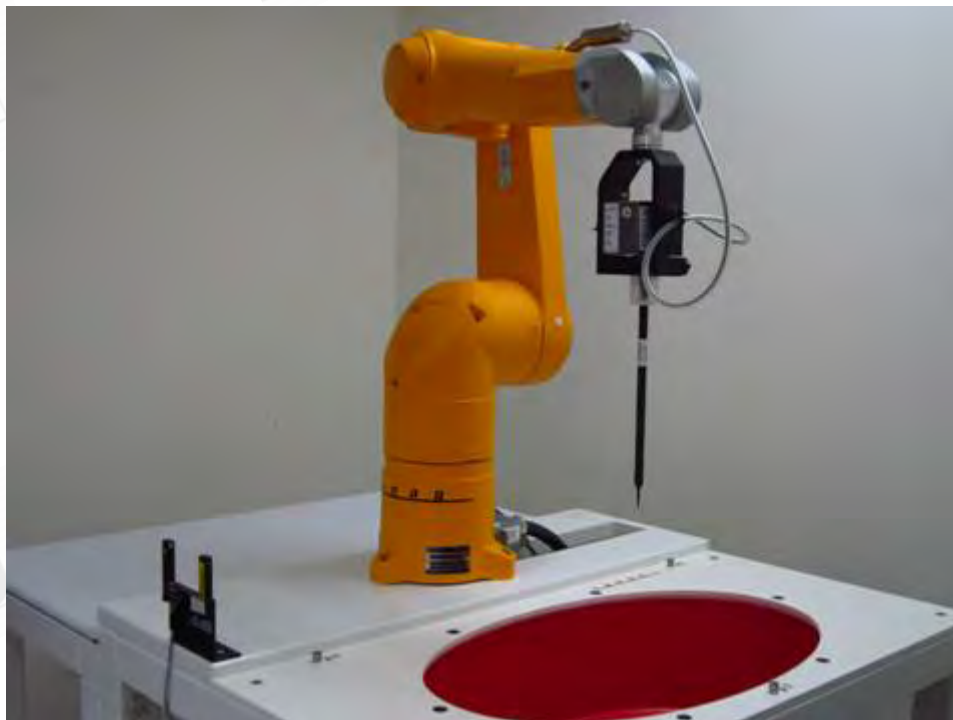
Fig.1 Photograph of the SAR measurement system
