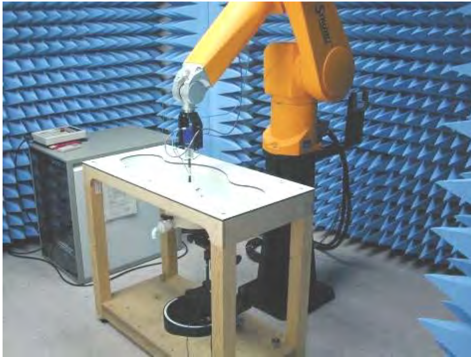
Fig.1 Photograph of the SAR measurement System
