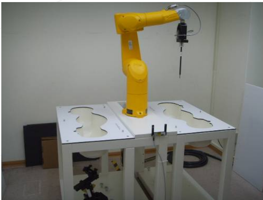
Fig.1 Photograph of the SAR measurement System
