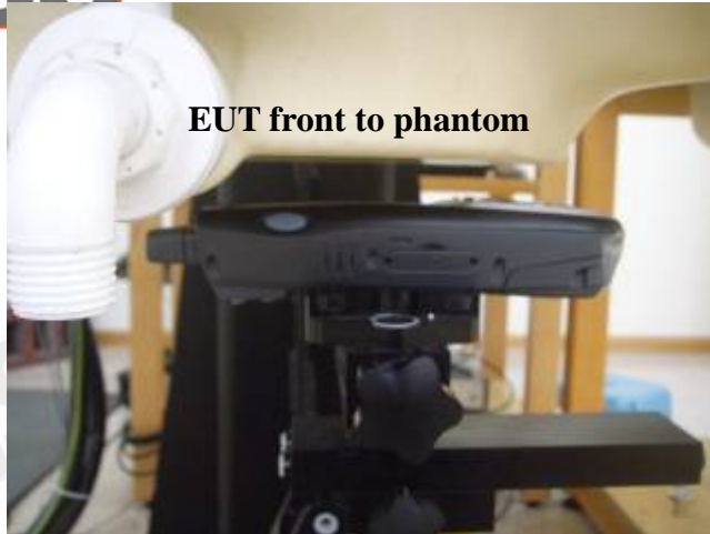
Fig.7 Body worn- EUT front to flat phantom and distance between flat phantom and mobile phone is 1.5 cm
