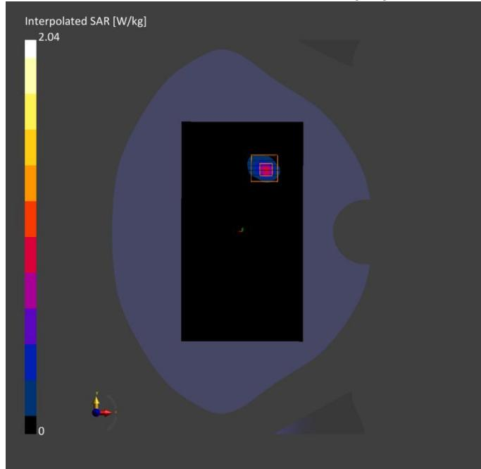
**Meas.18 Limb Plane with Back Side 0mm on 116 Channel in IEEE802.11a mode with Antenna 3**
