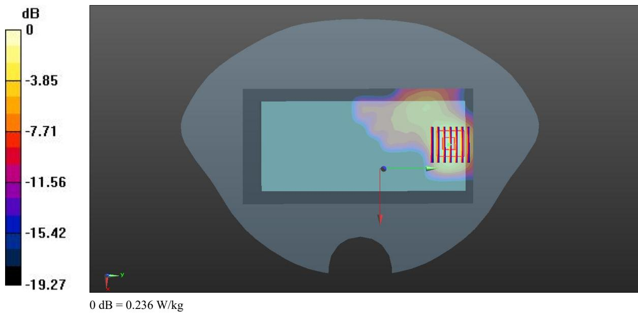
**Meas.13 Body Plane with Back Side 10mm on High Channel in LTE Band41 mode with Ant.0**
