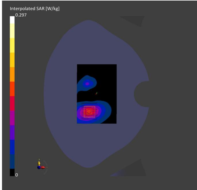
**Meas.17 Limb Plane with Back Side 0mm on 52 Channel in IEEE802.11a mode with Antenna 3**
