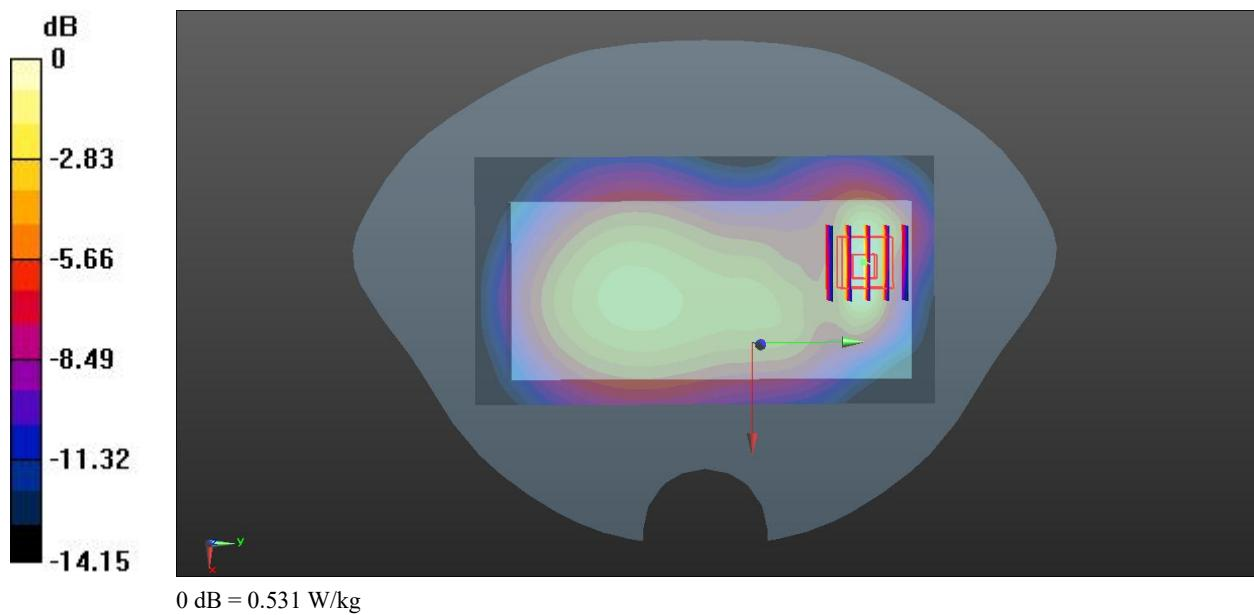
**Meas.5 Body Plane with Back Side 10mm on Low Channel in LTE Band2 mode with Ant.0**
