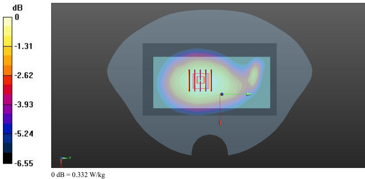
**Meas.10 Body Plane with Back Side 10mm on Middle Channel in LTE Band14 mode with Ant.0**
