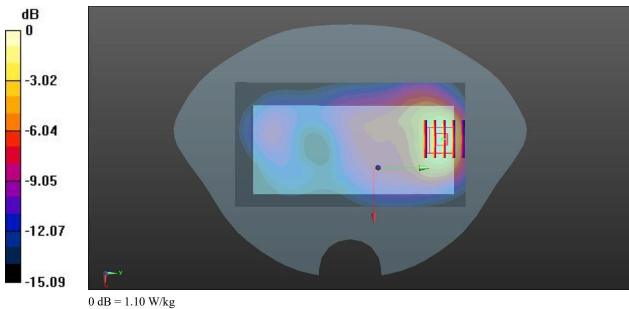
**Meas.3 Body Plane with Back Side 10mm on Middle Channel in WCDMA Band1 mode with Ant.0**
