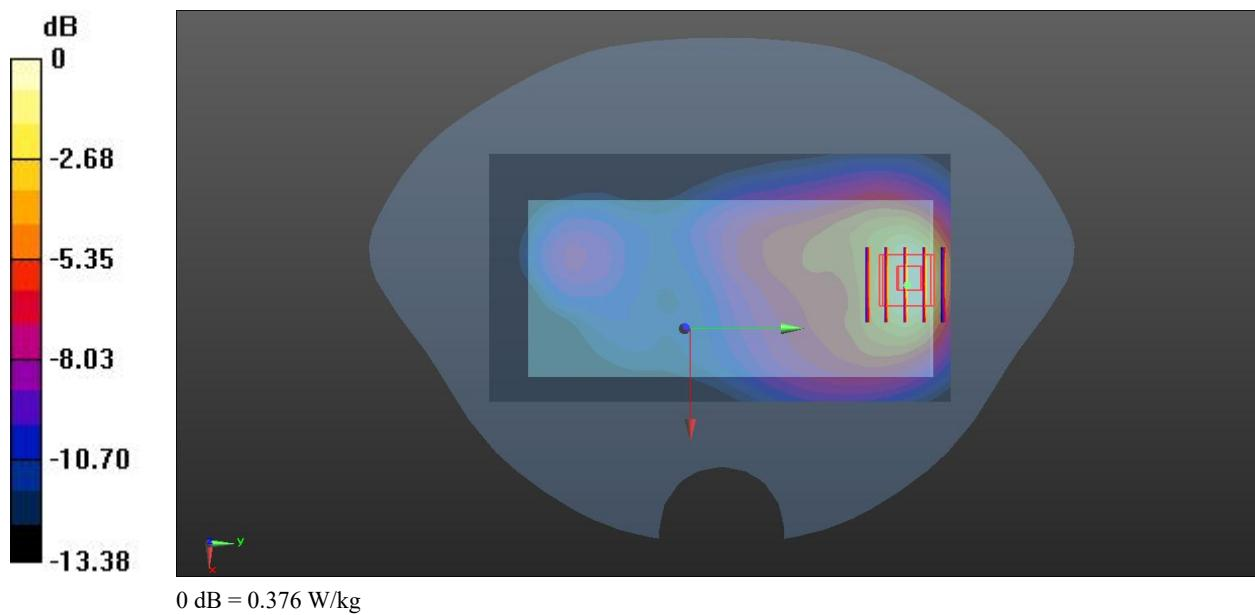
**Meas.7 Body Plane with Back Side 10mm on High Channel in LTE Band5 mode with Ant.0**
