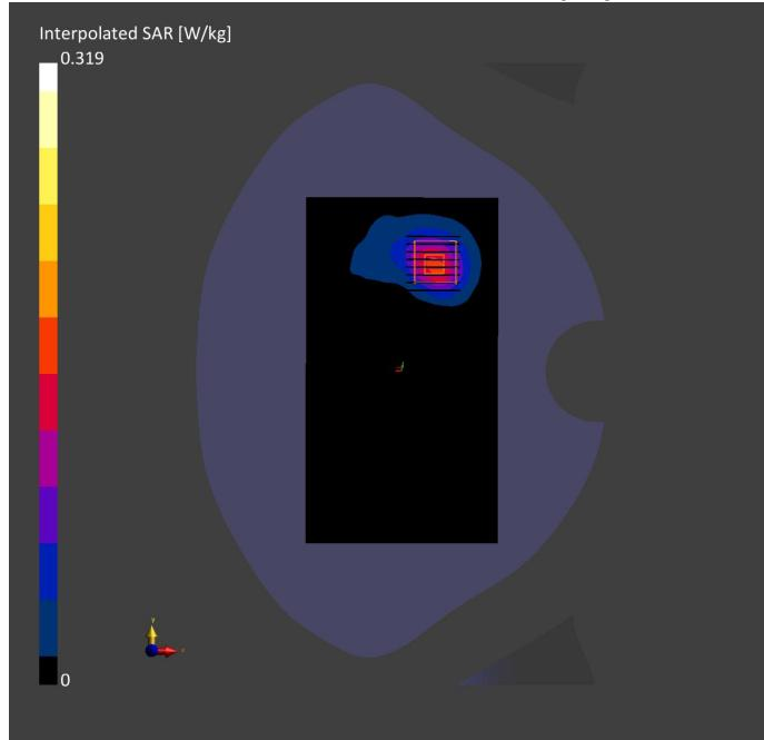
**Meas.16 Body Plane with Bottom Edge 10mm on 165 Channel in IEEE802.11a mode with Antenna 3**
