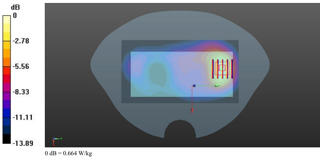
**Meas.4 Body Plane with Back Side 10mm on Middle Channel in WCDMA Band5 mode with Ant.0**
