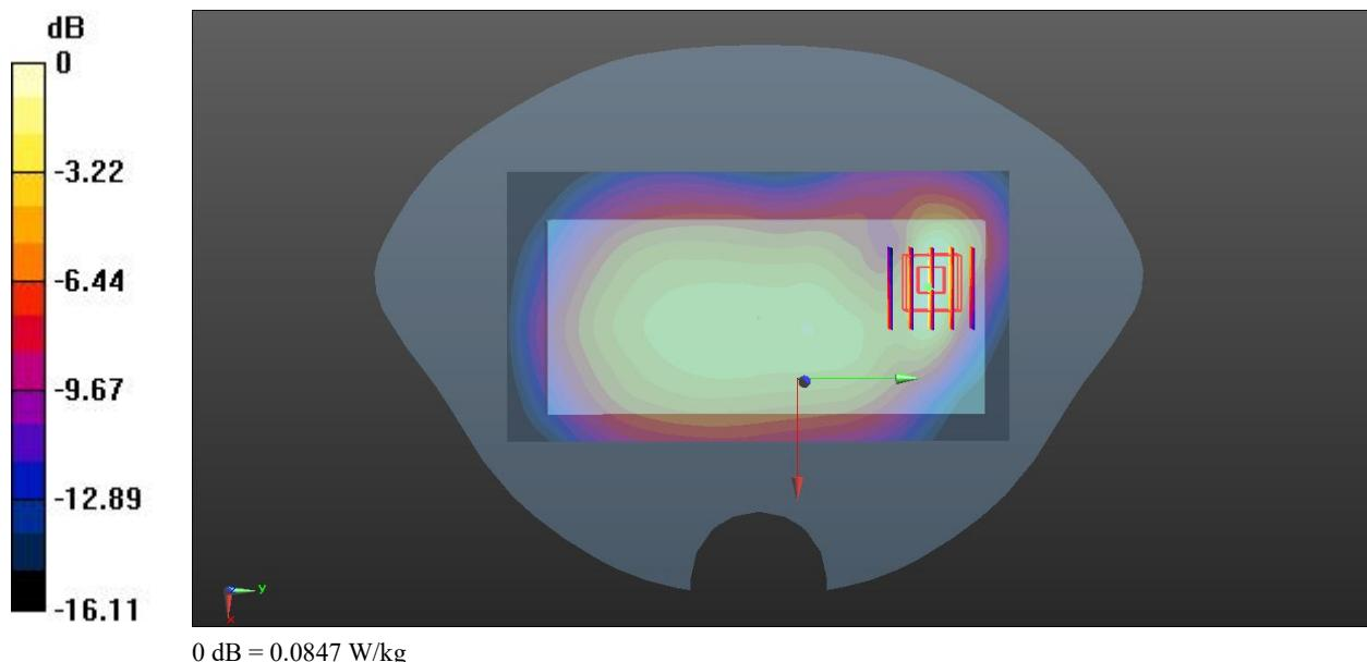
**Meas.11 Body Plane with Back Side 10mm on Middle Channel in LTE Band17 mode with Ant.0**
