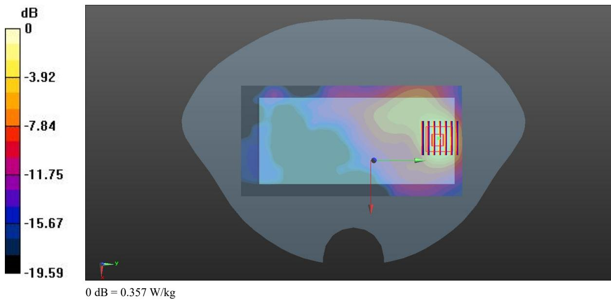
**Meas.14 Body Plane with Back Side 10mm on 1 Channel in IEEE802.11b mode with Ant.2**
