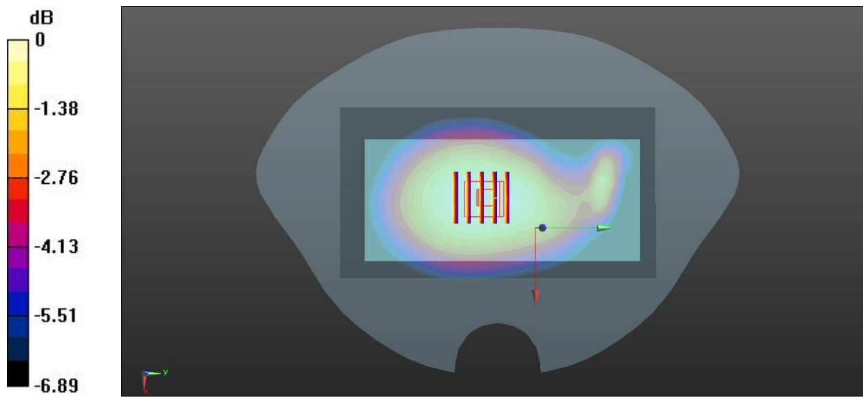
**Meas.12 Body Plane with Back Side 10mm on High Channel in LTE Band38 mode with Ant.0**
