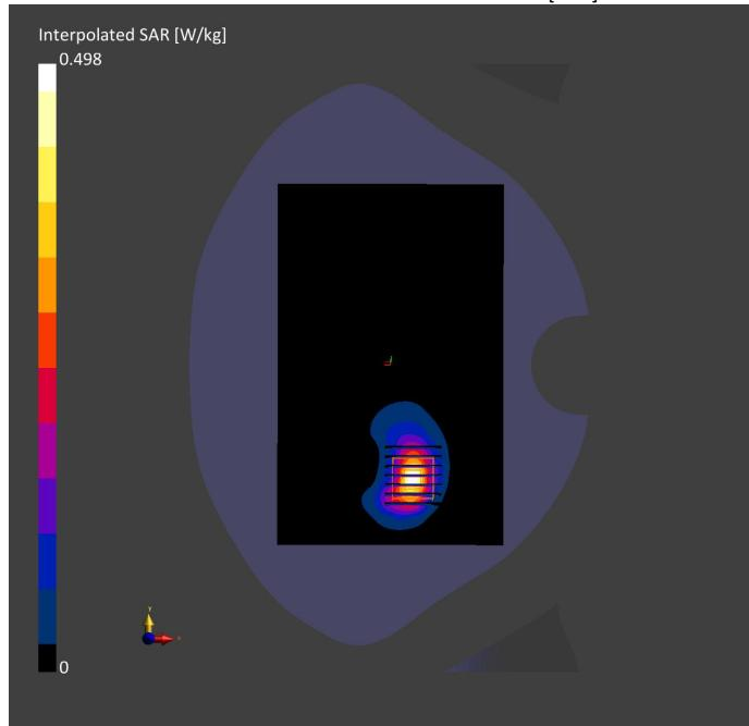
**Meas.15 Body Plane with Back Side 10mm on 44 Channel in IEEE802.11a mode with Antenna 3**
