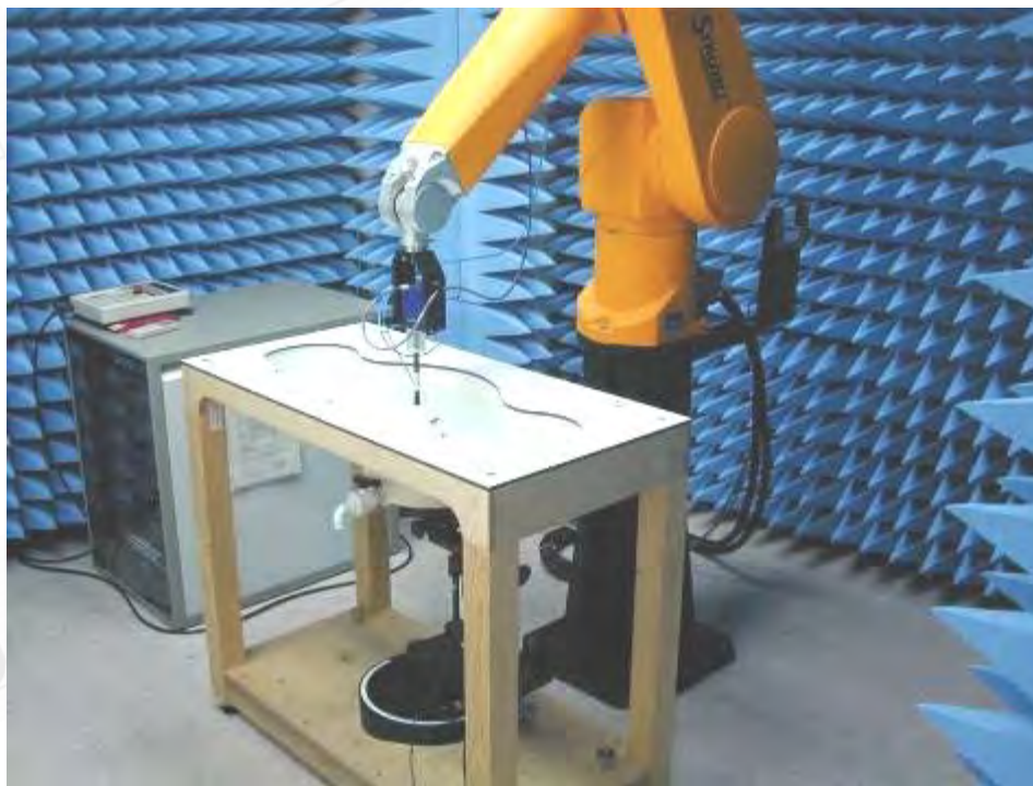
Fig.1 Photograph of the SAR measurement System
