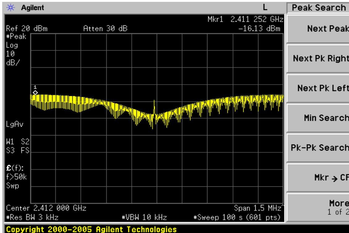
**Copyright 2000-2005 Agilent Technologies****Power Spectral Density Test Plot (CH-Mid)**
