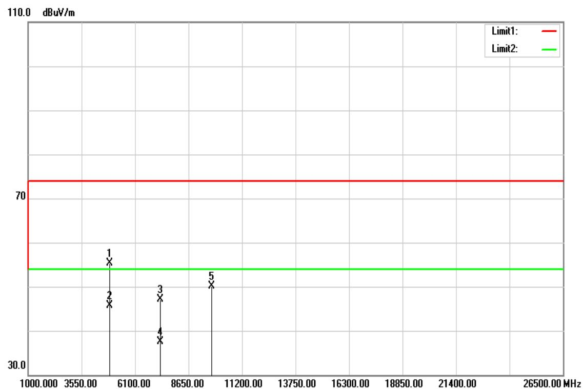
**Operation Mode:** TX / GFSK / DH5 / CH Mid**Test Date:** October 4, 2016**Temperature:** 26°C**Tested by:** Dennis Li**Humidity:** 50 % RH**Polarity:** Ver. / Hor.
