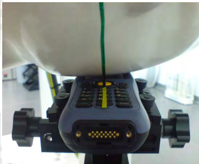
Fig.5 Left Head Section / Cheek-Touch Position
