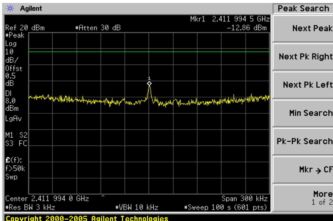
**Power Spectral Density Test Plot (CH-Mid)**
