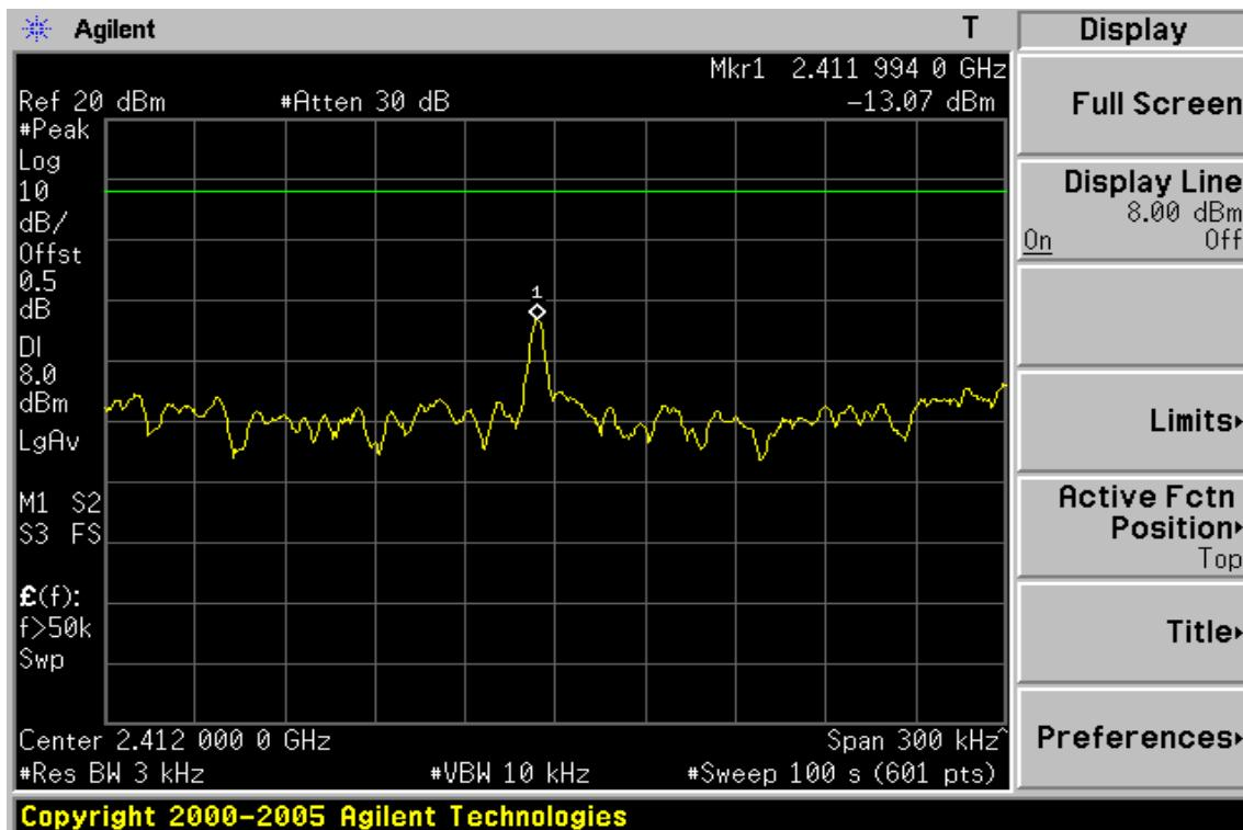
**Power Spectral Density Test Plot (CH-Mid)**
