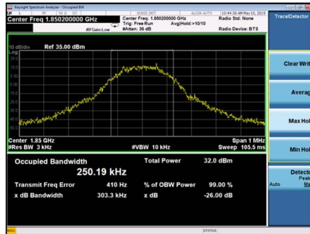
(Plot D1: EDGE 1900MHz Channel = 512 Occupied bandwidth)
