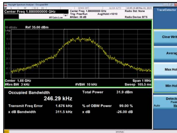
(Plot D2: EDGE 1900MHz Channel = 661 Occupied bandwidth)
