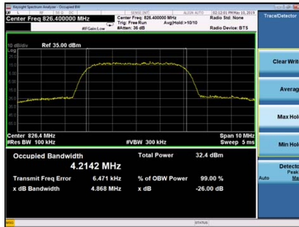
(Plot E1: WCDMA 850MHz Channel = 4132 Occupied bandwidth)
