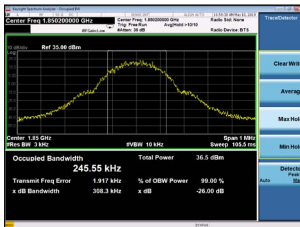
(Plot B1: GSM 1900MHz Channel = 512 Occupied bandwidth)
