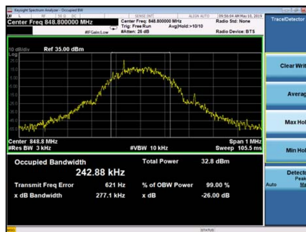
(Plot C3: EDGE 850MHz Channel = 251 Occupied bandwidth)
