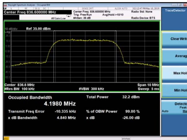
(Plot E2: WCDMA 850MHz Channel = 4183 Occupied bandwidth)
