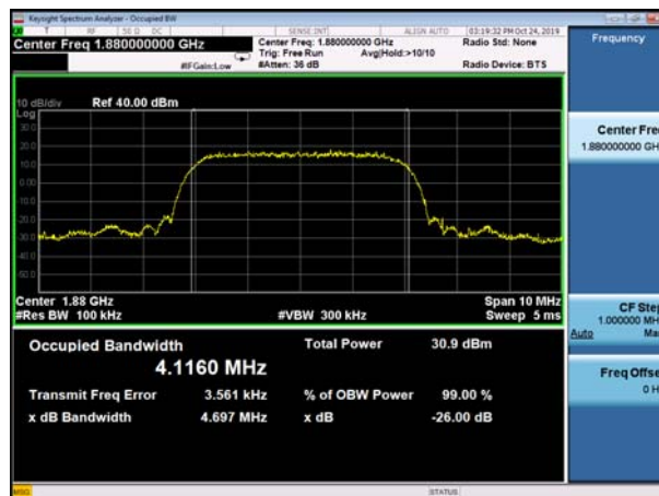
(Plot F2: WCDMA 1900MHz Channel = 9400 Occupied bandwidth)
