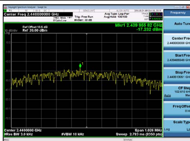
Power spectral density: 2440MHz
