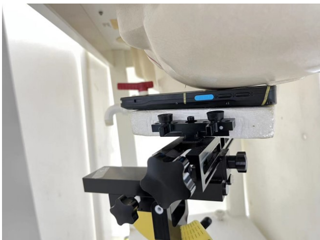
Left Cheek, Test Separation 0 mm
