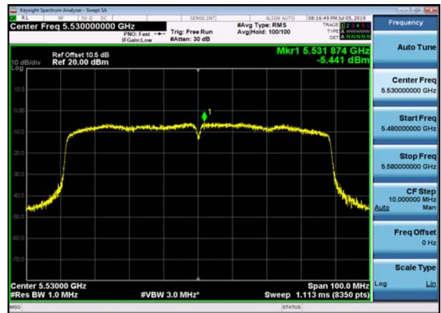
U-NII-2c Power spectral density-802.1 1ac(80MHz),5530MHz,Ant1
