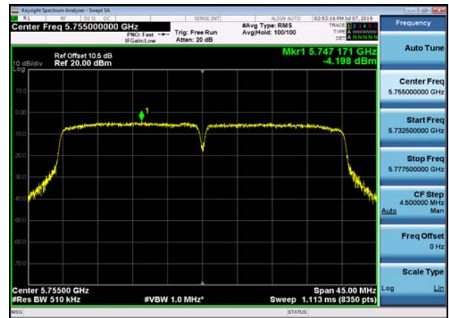
U-NII-3 Power spectral density-802.11 a(20MHz),5745MHz,Ant1
