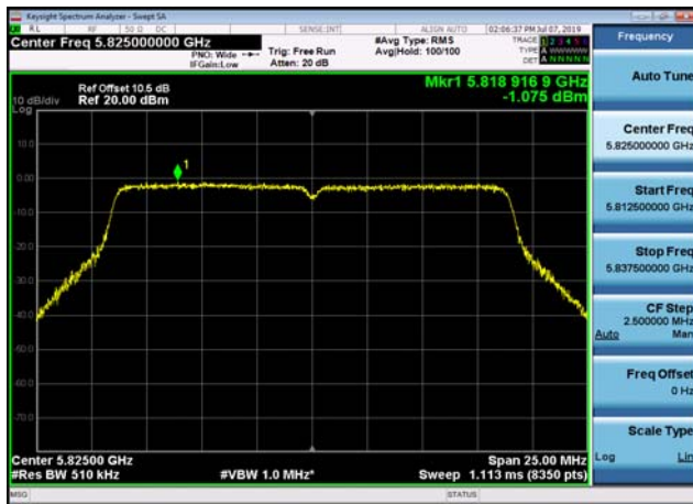
U-NII-3 Power spectral density-802.11 n(40MHz),5795MHz,Ant1
