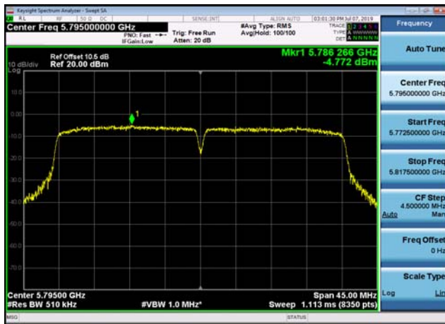
U-NII-3 Power spectral density-802.11 a(20MHz),5785MHz,Ant1
