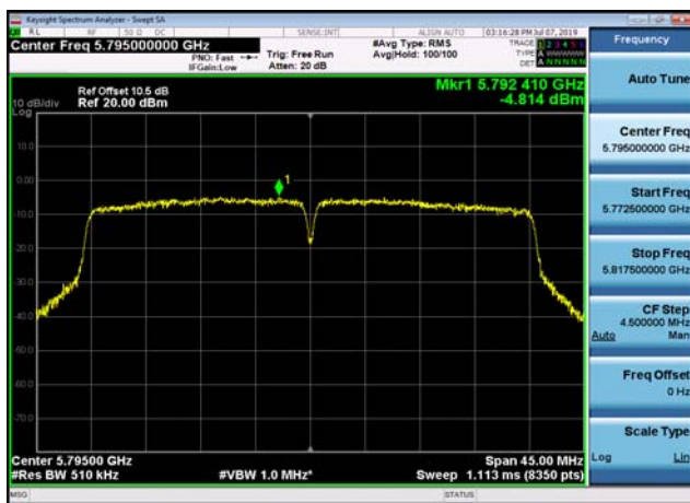
U-NII-3 Power spectral density-802.11 ac(40MHz),5795MHz,Ant1
