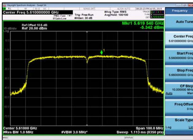
U-NII-3 Power spectral density-802.11 n(20MHz),5745MHz,Ant1
