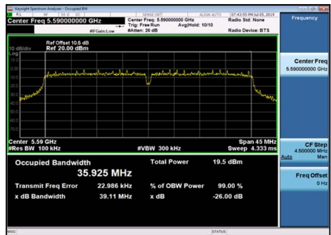
U-NII-2c 26dB Bandwidth-802.11ac(80MHz),5530MHz,Ant1
