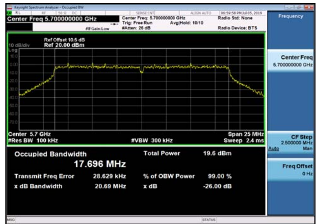
U-NII-2c 26dB Bandwidth-802.11ac(40MHz),5590MHz,Ant1
