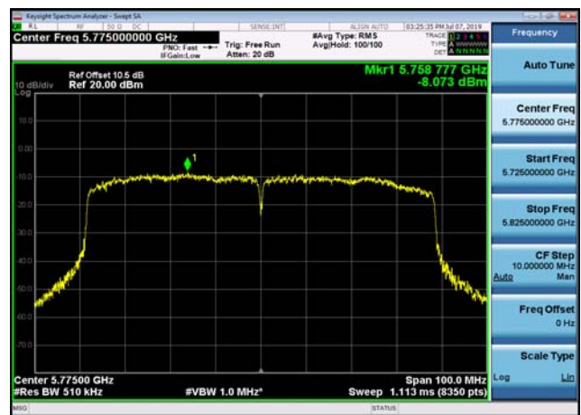
U-NII-3 Power spectral density-802.11 ac(80MHz),5775MHz,Ant1
