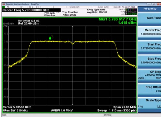
U-NII-3 Power spectral density-802.11 a(20MHz),5785MHz,Ant1
