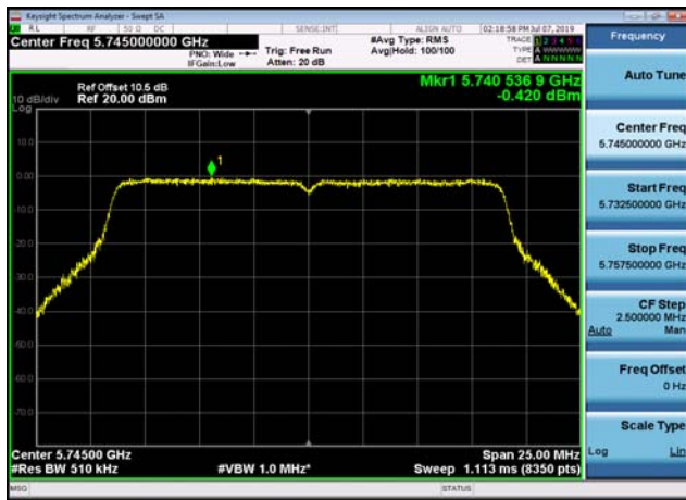
U-NII-3 Power spectral density-802.11 ac(20MHz),5825MHz,Ant1
