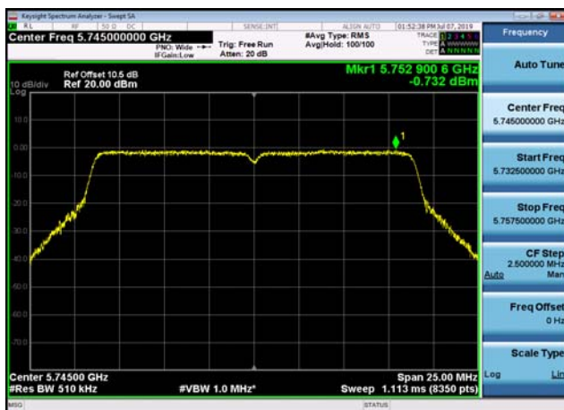
U-NII-3 Power spectral density-802.11 n(20MHz),5745MHz,Ant1
