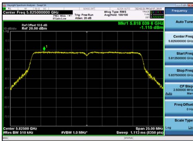
U-NII-3 Power spectral density-802.11 ac(40MHz),5795MHz,Ant1
