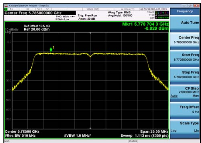
U-NII-3 Power spectral density-802.11 n(20MHz),5785MHz,Ant1
