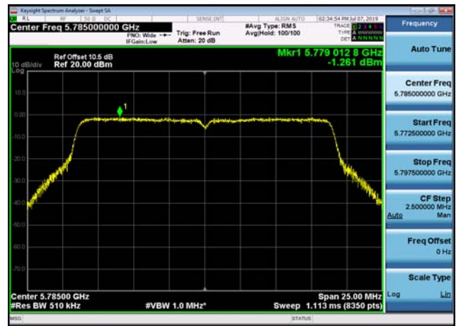
U-NII-3 Power spectral density-802.11 ac(40MHz),5755MHz,Ant1
