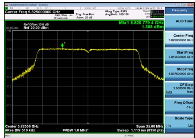
U-NII-3 Power spectral density-802.11 a(20MHz),5825MHz,Ant1
