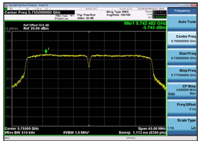
U-NII-3 Power spectral density-802.11 ac(80MHz),5775MHz,Ant1
