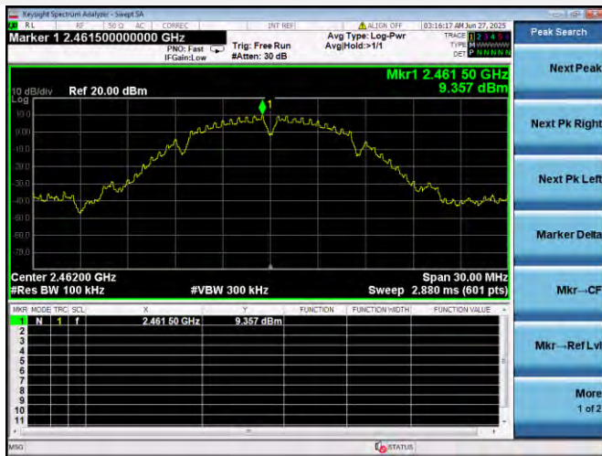
802.11b HIGH CHANNEL, CARRIER LEVEL
