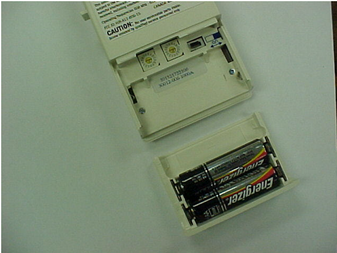
Photo Six Battery Pack Removed to Expose Programming Switches
