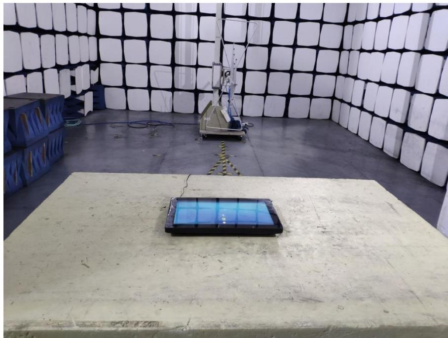
**Radiation Emission Test Setup (1GHz to 18GHz)**
