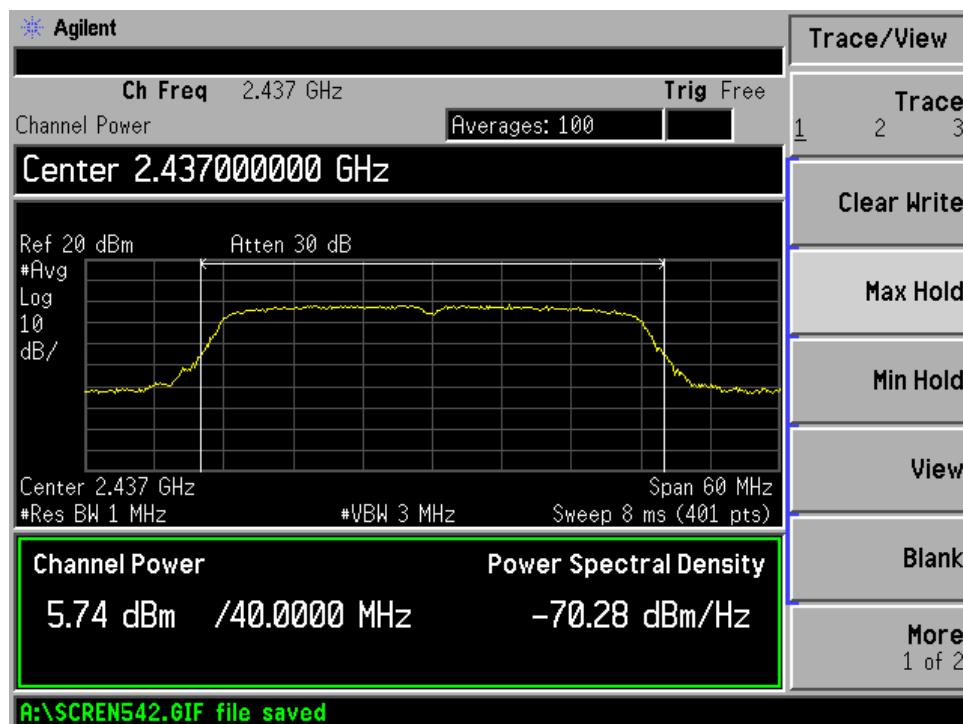
Result data graph shows high channel conducted power = 5.53dBm
