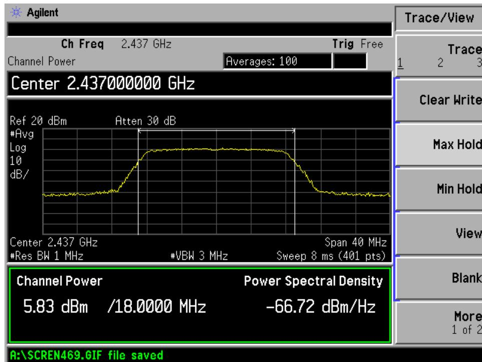
Result data graph shows high channel conducted power = 5.03dBm
