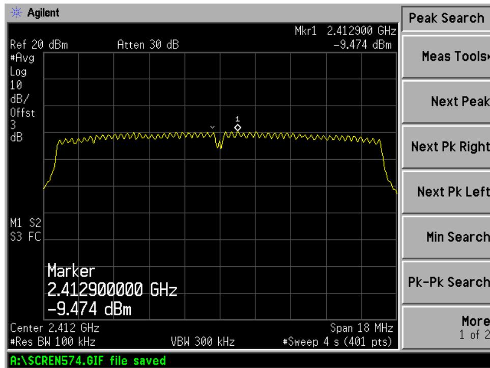
Result data graph shows middle channel power spectrum density is -10.38dBm at 100kHz RBW
