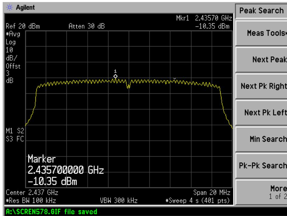
Result data graph shows high channel power spectrum density is -11.49dBm at 100kHz RBW
