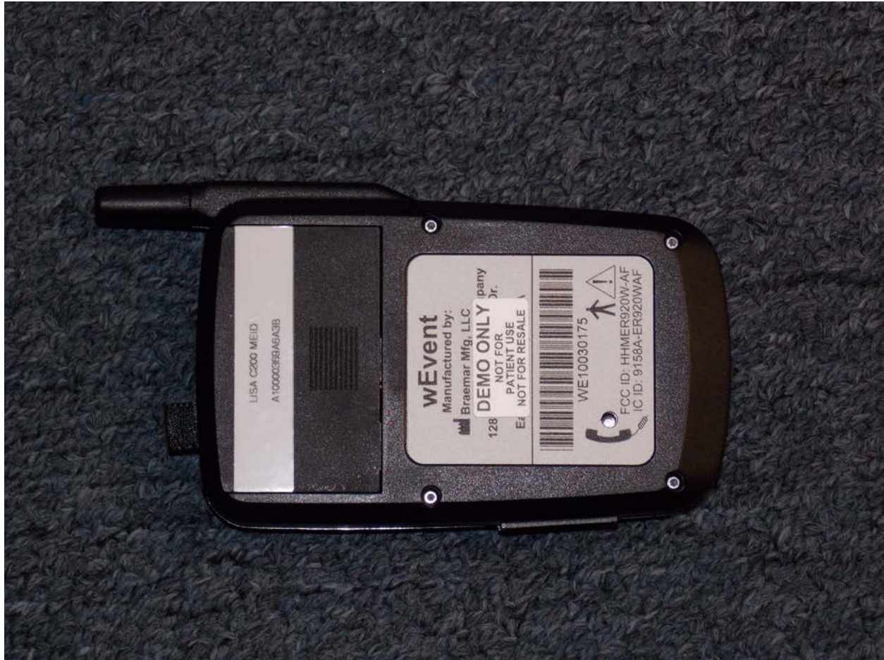
Back of Device (This was a modified device where a CDMA module was put in a 2G device. The FCC ID is not the correct ID for this model)
