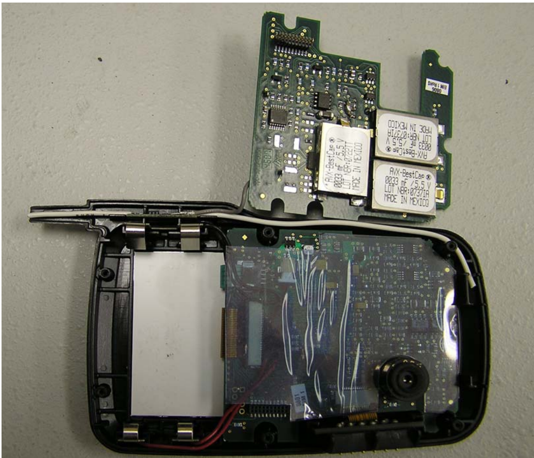
EUT - Cell modem and ER920 boards
