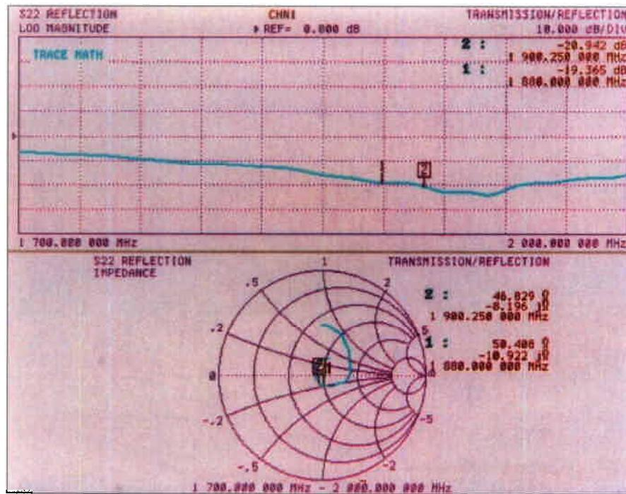
Dipole impedance at 1900 MHz  $\text{Re}\{Z\} = 46.8 \Omega$
