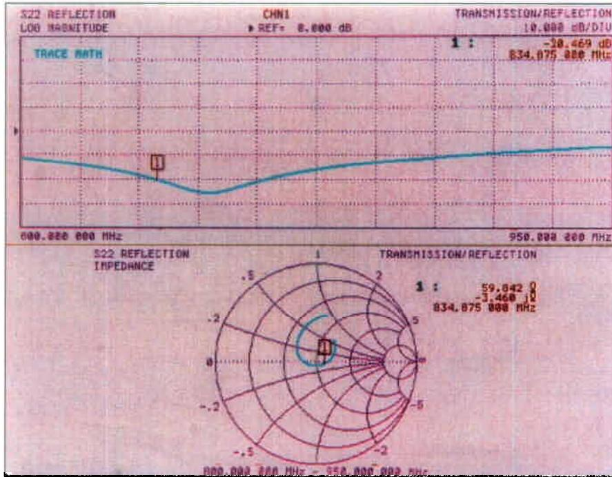
Dipole impedance at 835 MHz       $\text{Re}\{Z\} = 59.8 \Omega$
