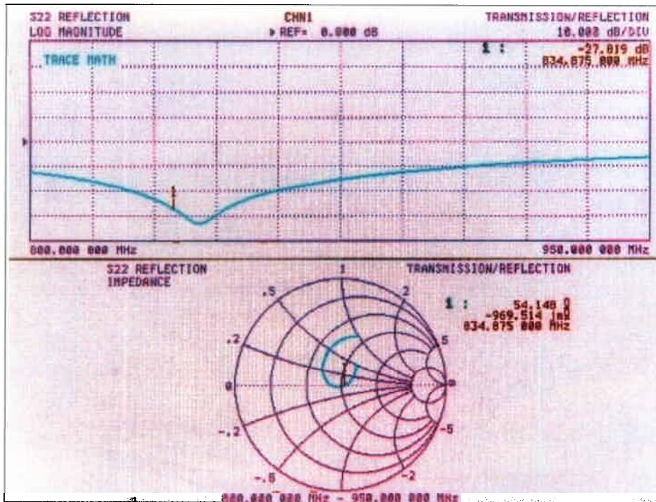
Dipole impedance at 835 MHz       $\text{Re}\{Z\} = 54.1 \Omega$
