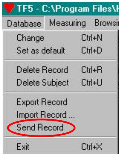
Then, select/mark the record to be sent - simply by moving the arrow at the left/hand side of the basic database screen (name of the subject in the upper part of the screen, individual record/s in the lower part). Afterwards, selected HRV data can be sent via a standard e-mail program (MS Outlook) by choosing option **Database** -> **Send Record**. Whenever connected to Internet, the data will be automatically sent to the address indicated in the Setup.
