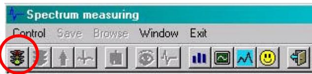
(g) Note that -- when properly started - **Icons setting** changes consistently, i.e., Start icon is disabled and Stop icon along with other icons related to current program step are enabled. The same is valid for **Measuring Control buttons** at the window bottom (Start, Stop, Save, Browse and ECG).
