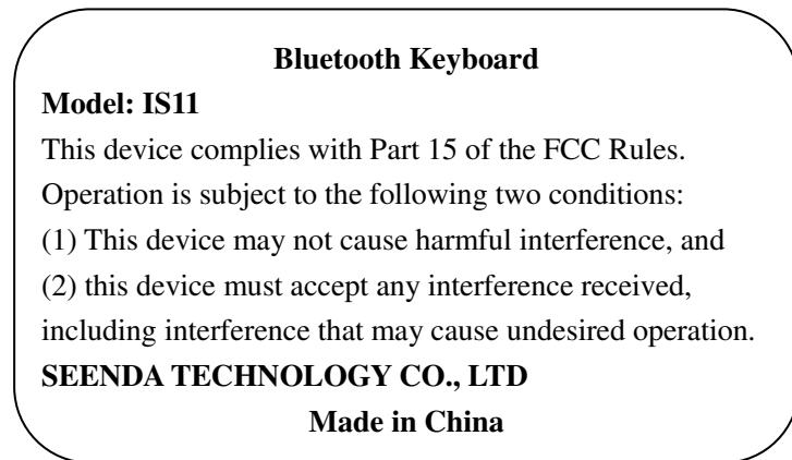
Specifications: Text is Black in color and justified. Labels are printed in indelible ink on permanent adhesive silk-screened onto the EUT or shall be affixed at a conspicuous location on the EUT.
