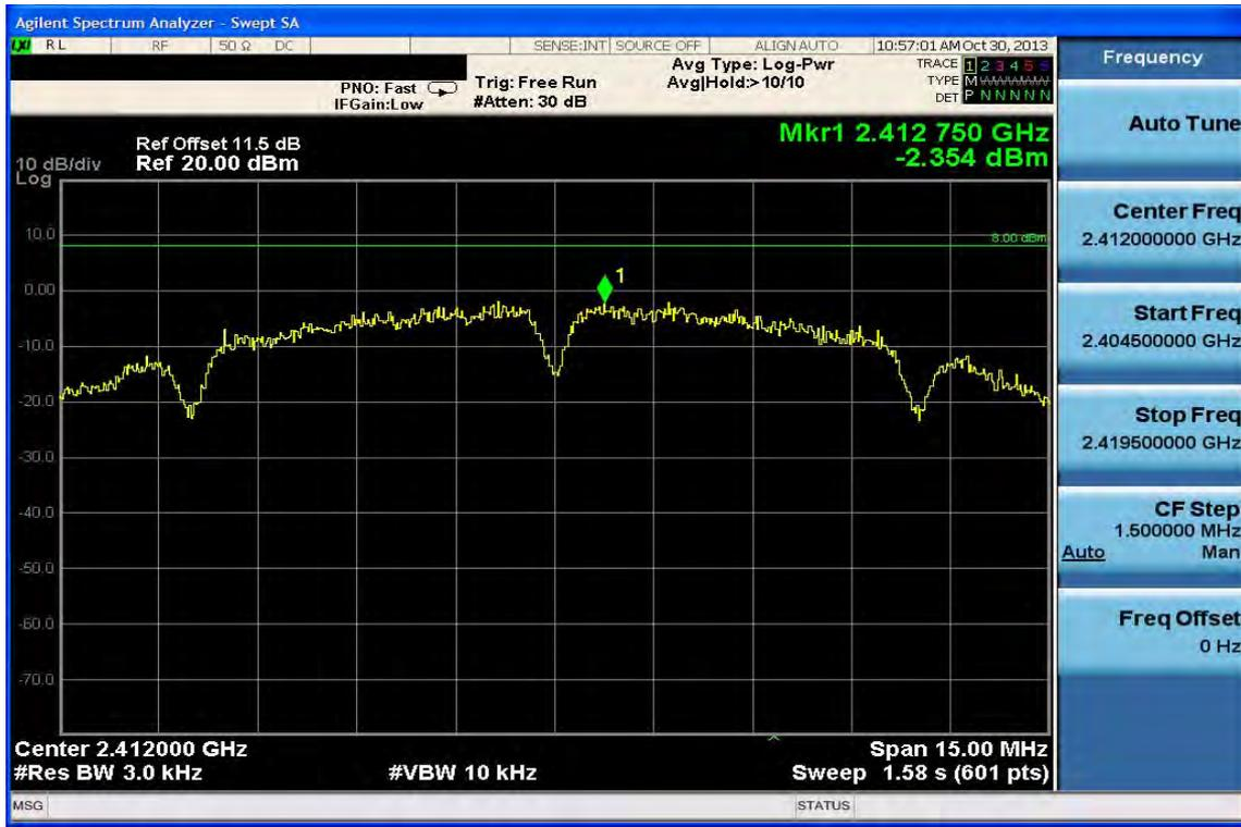
Power Spectral Density Test Plot (CH-Mid)
