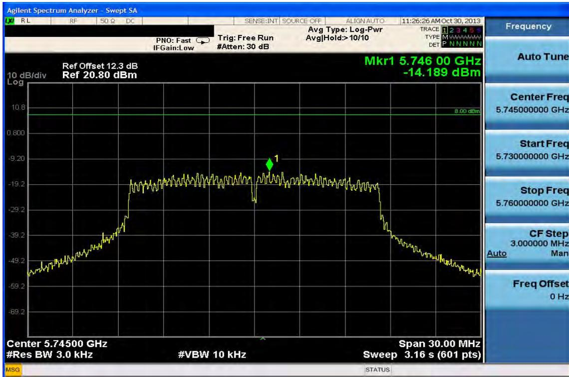
Power Spectral Density Test Plot (CH-Mid)
