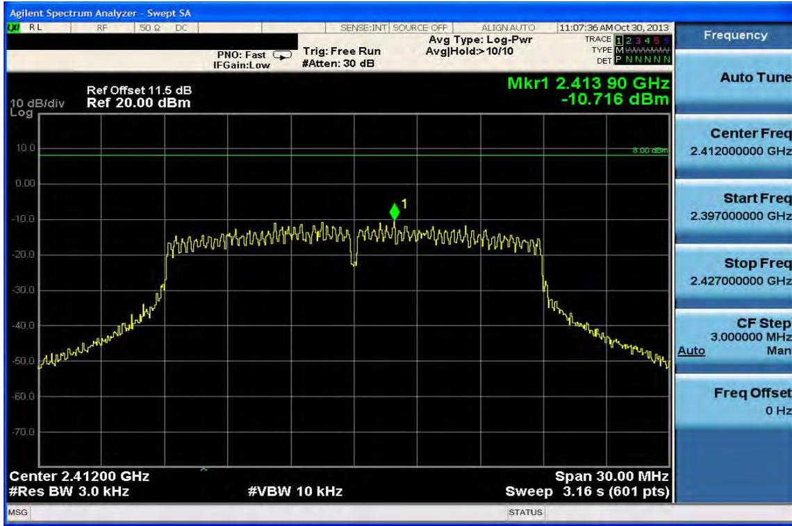
Power Spectral Density Test Plot (CH-Mid)
