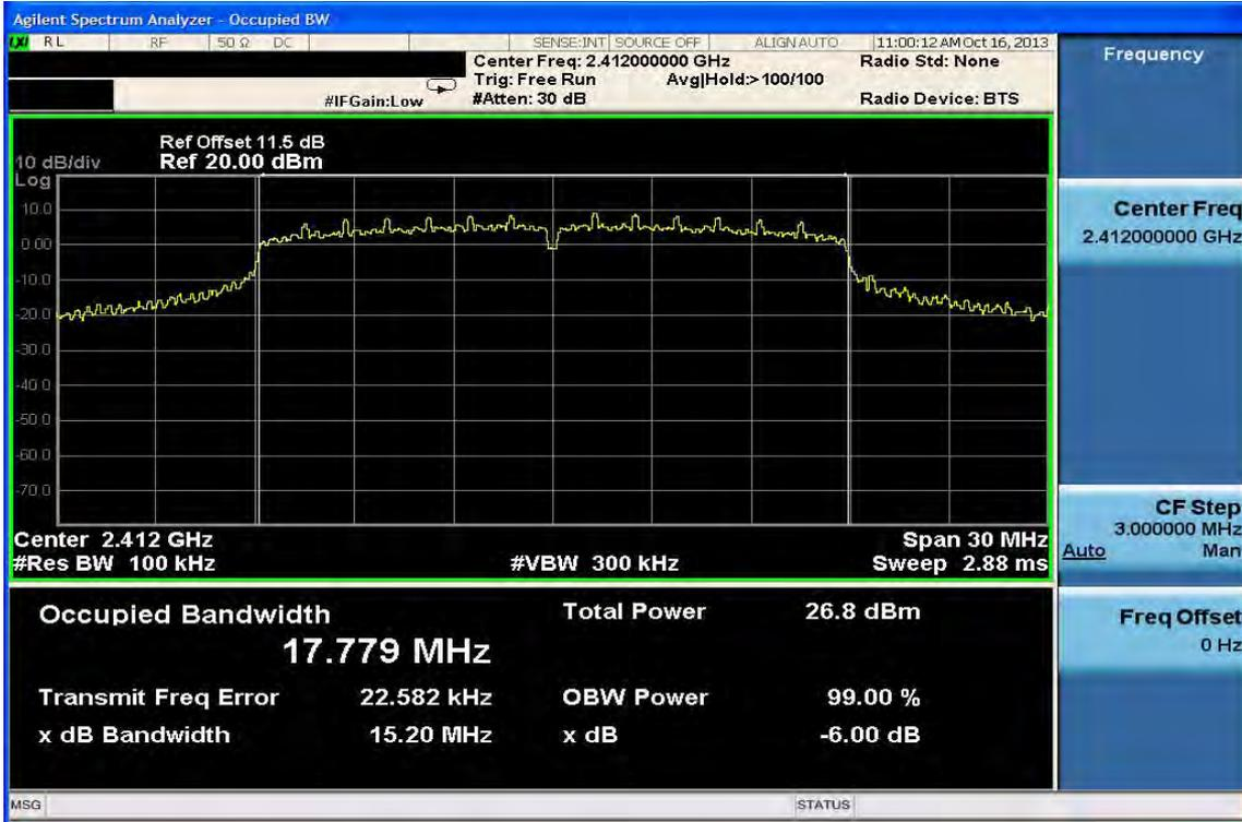
6dB Band Width Test Data CH-Mid
