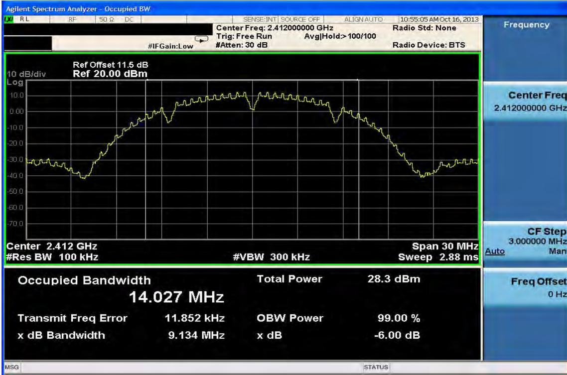
6dB Band Width Test Data CH-Mid
