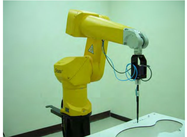
Fig. 5.2 Probe setup on robot
