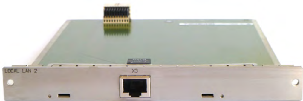
Figure 3-25: Local LAN2 Board
