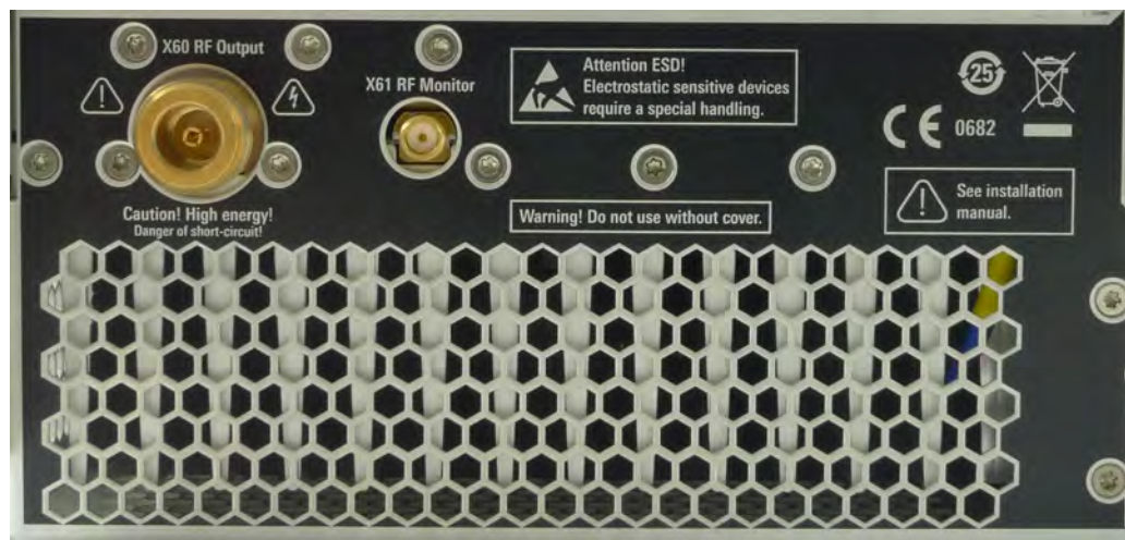
Figure 3-34: RF output and RF monitor connectors on rear panel of R&S TLx9
