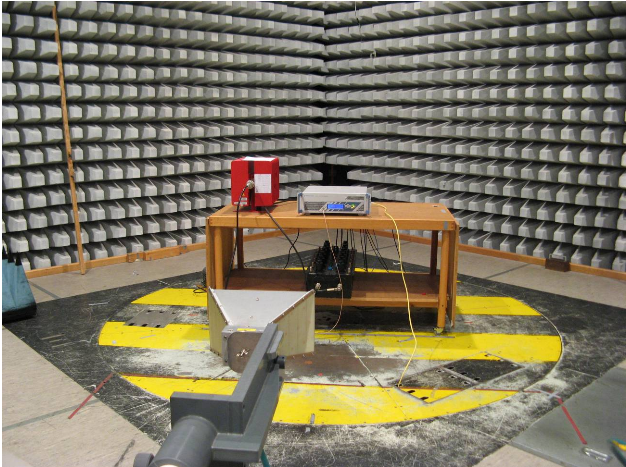
Figure 6-4: Test setup for radiated emission measurement, 1 - 10GHz
