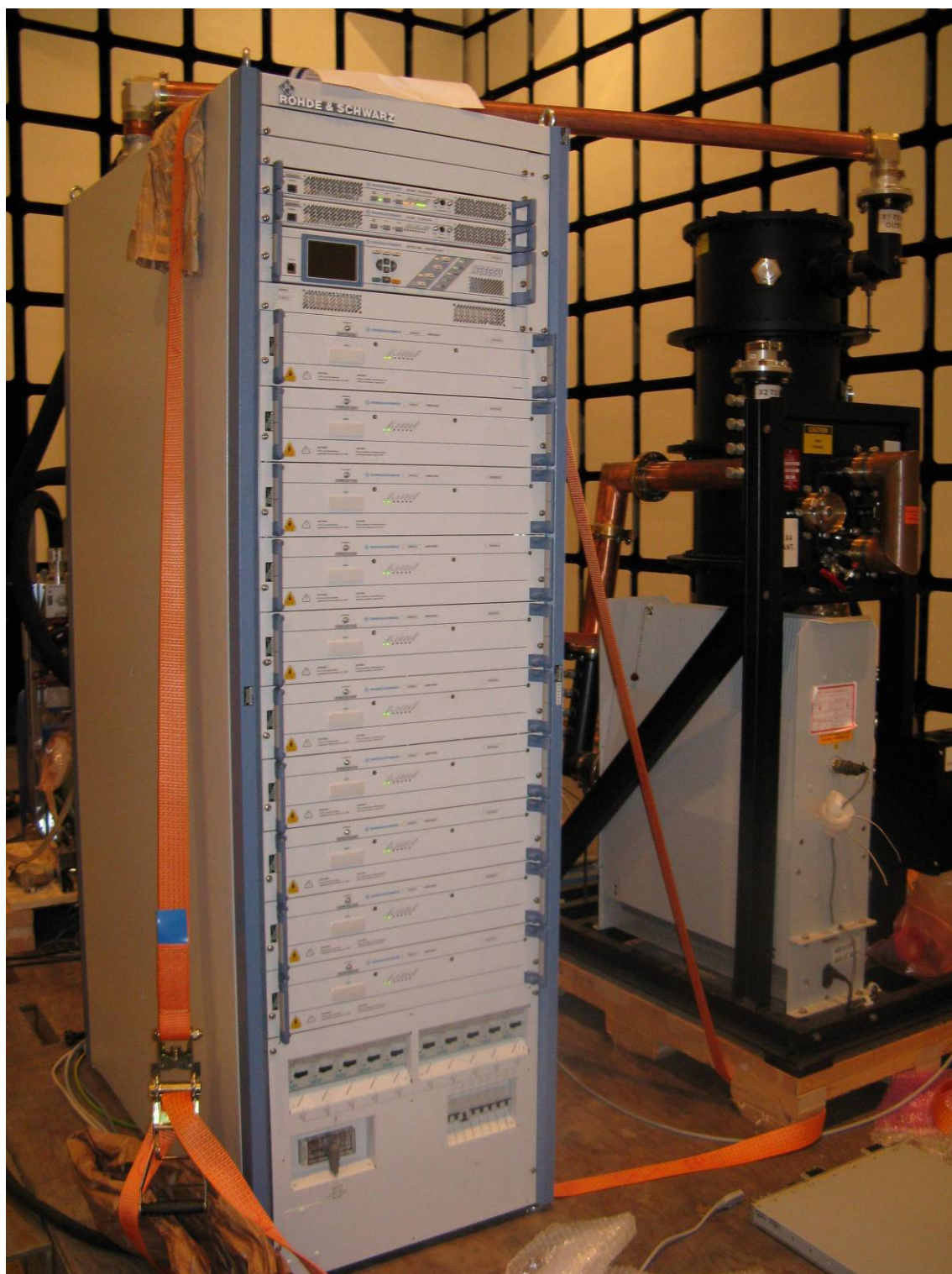
Figure 4-3: NV8610V in the EMC chamber for Emission Tests
