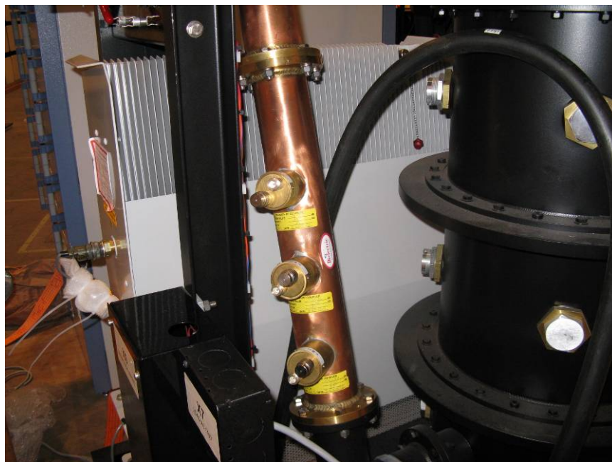
Figure 6-8: Picture of Power Coupler
