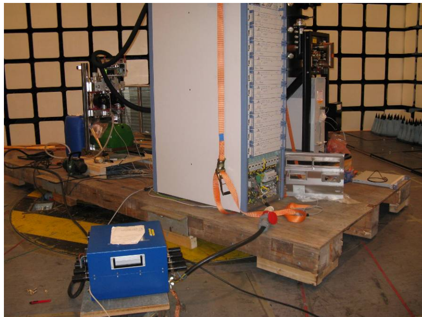
Figure 6-15: Test setup for conducted emissions measurement
