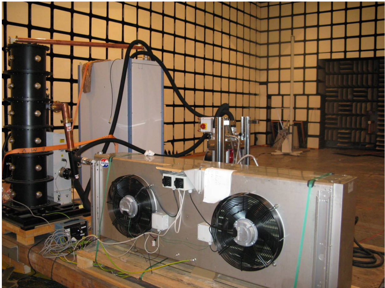
Figure 6-2: Test setup for radiated emissions measurement
