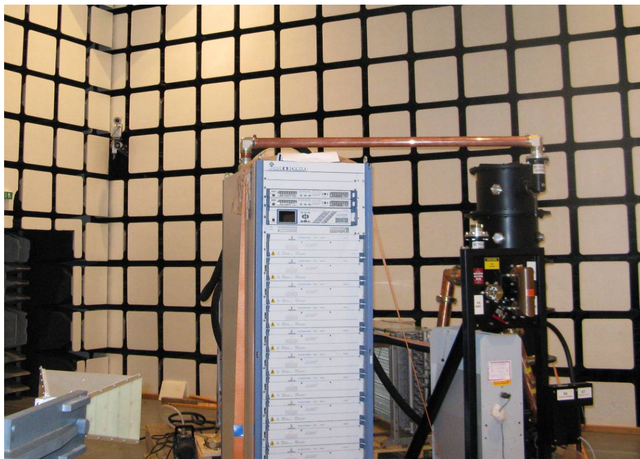
Figure 6-4: Test setup for radiated emission measurement, 1 - 10GHz
