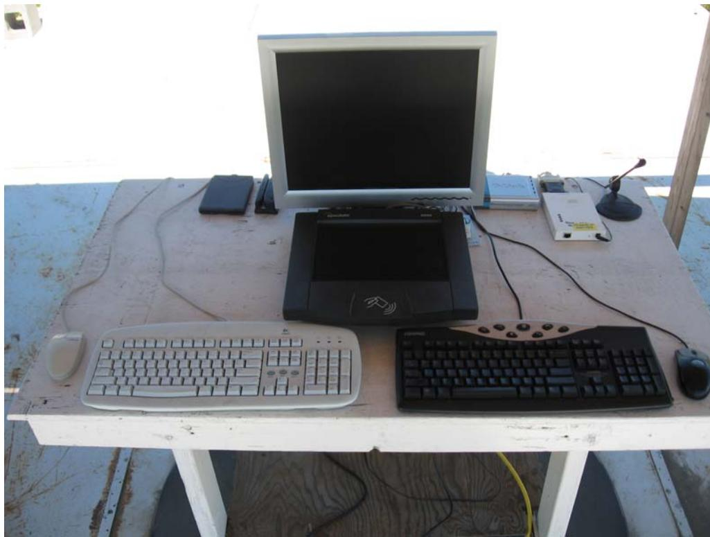
**- Test configuration for Conducted Emission**
