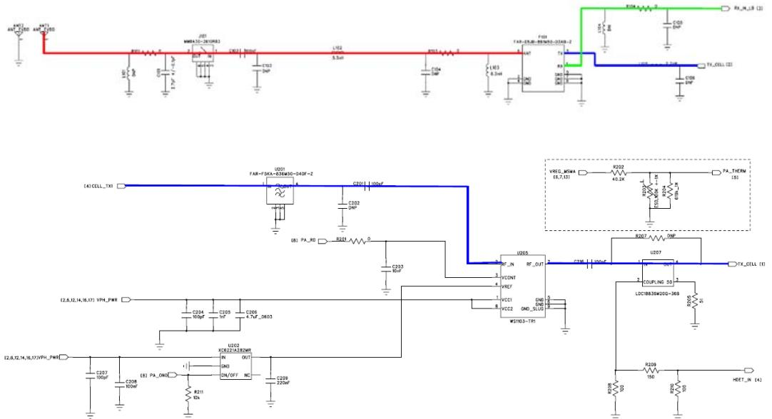
**Receiving:** The received signal is fed in through the antenna and duplexer, and is amplified by internal LNA, filtered by balun filter and then directly down-converted from RF to baseband. Before demodulation, the signal should be filtered, amplified and converted from analog signal to digital signal
