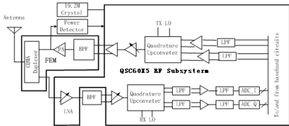
**Transmission:** The transmit signal is directly up-converted from the baseband to RF, and amplified by the VGA, then amplified by the PA, and finally radiated by the antenna.
