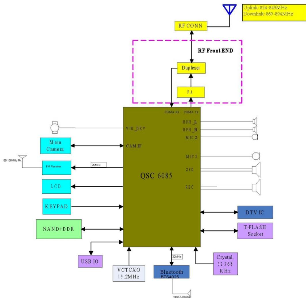
E3240 is based on the Qualcomm QSC6085-1 platform, with the following components.
