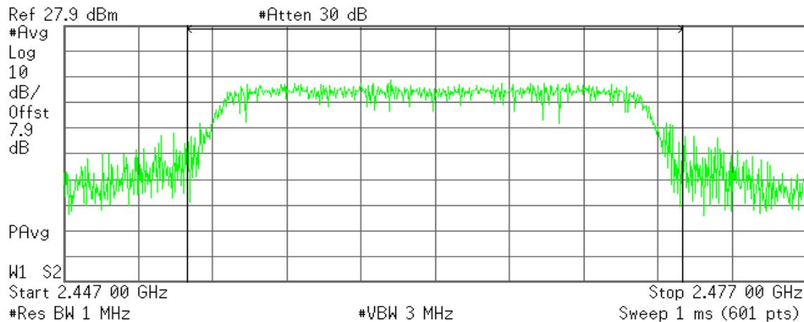
**Channel Power****14.35 dBm /20.0000 MHz****Power Spectral Density****-58.66 dBm/Hz**
