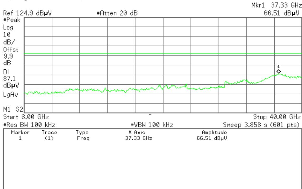
**IEEE 802.11a Base mode / CH High****30MHz ~ 8GHz****\* Agilent 19:04:22 Sep 11, 2004**
