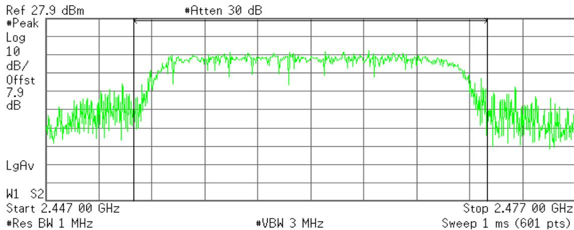
**Channel Power****17.78 dBm /20.0000 MHz****Power Spectral Density****-55.23 dBm/Hz****Peak power (CH 2462-Average)****Agilent** 20:28:05 Sep 16, 2004
