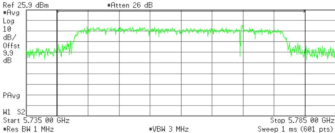
**Channel Power****20.89 dBm /40.0000 MHz****Power Spectral Density****-55.13 dBm/Hz**
