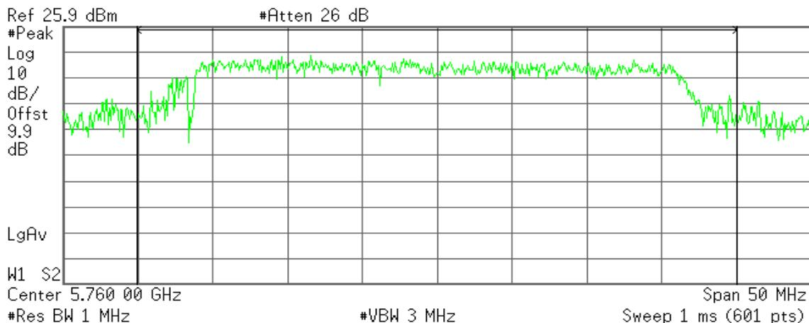
**Channel Power****24.50 dBm /40.0000 MHz****Power Spectral Density****-51.52 dBm/Hz****Peak power (CH 5760-Average)****Agilent 00:26:13 Sep 17, 2004**
