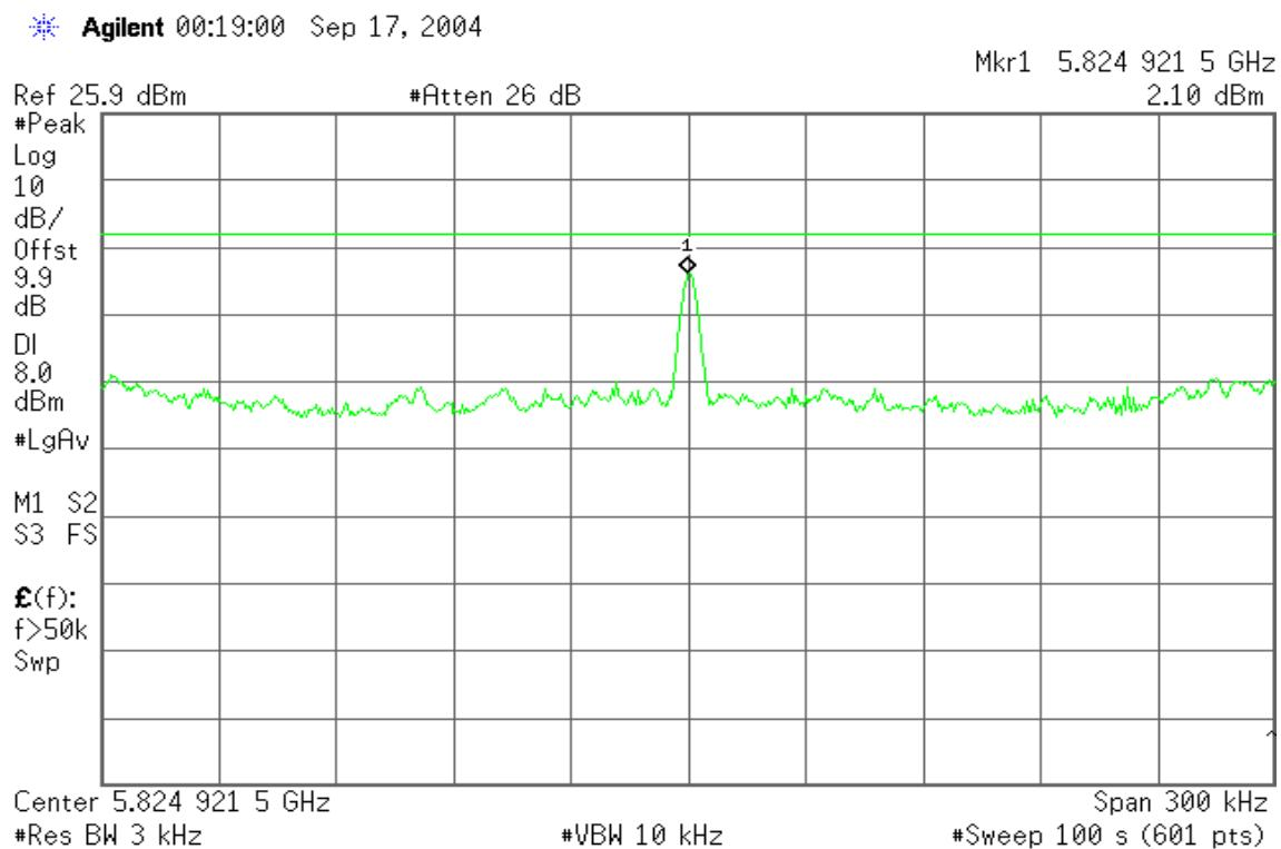
**IEEE 802.11a Turbo mode****PPSD (CH 5760)**
