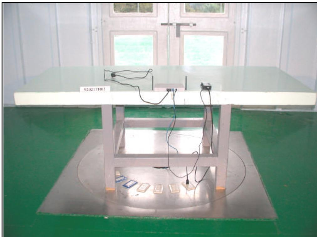
RADIATED EMISSION TEST (With POE)
