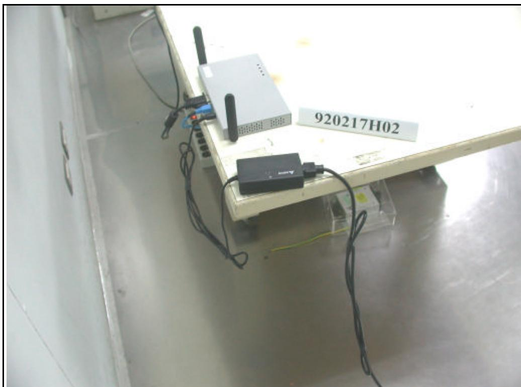
RADIATED EMISSION TEST (With Adapter)
