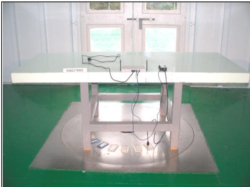
RADIATED EMISSION TEST (With POE)
