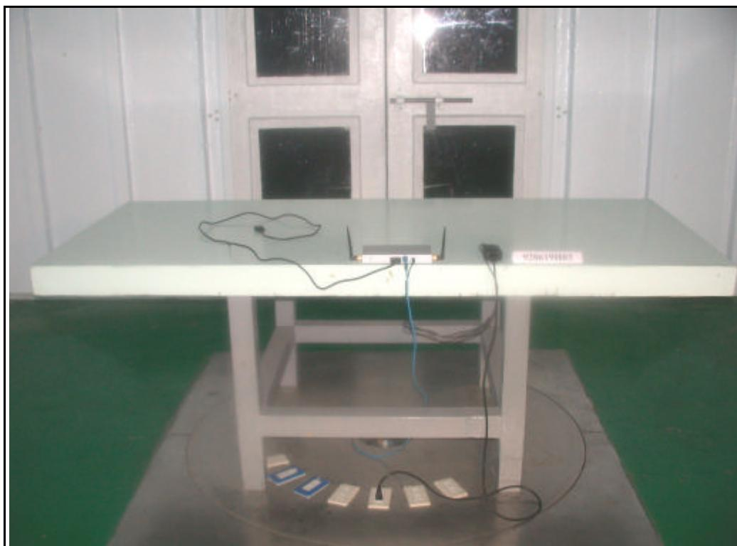
RADIATED EMISSION TEST (With POE)
