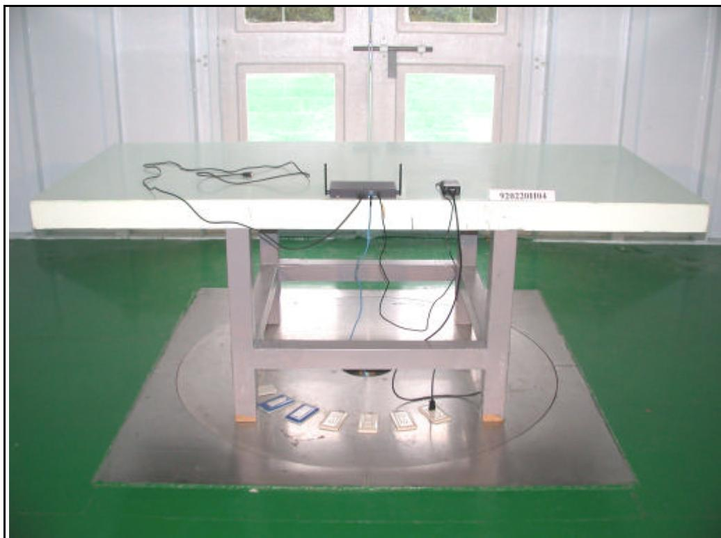
RADIATED EMISSION TEST (With POE)
