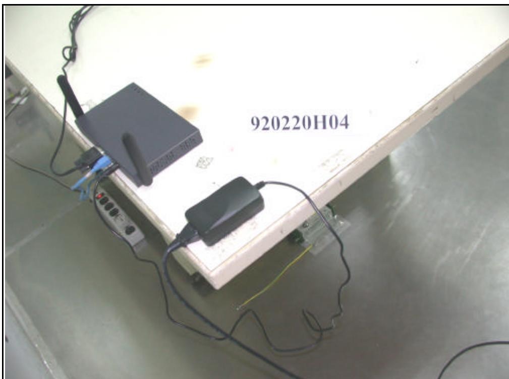
RADIATED EMISSION TEST (With Adapter)
