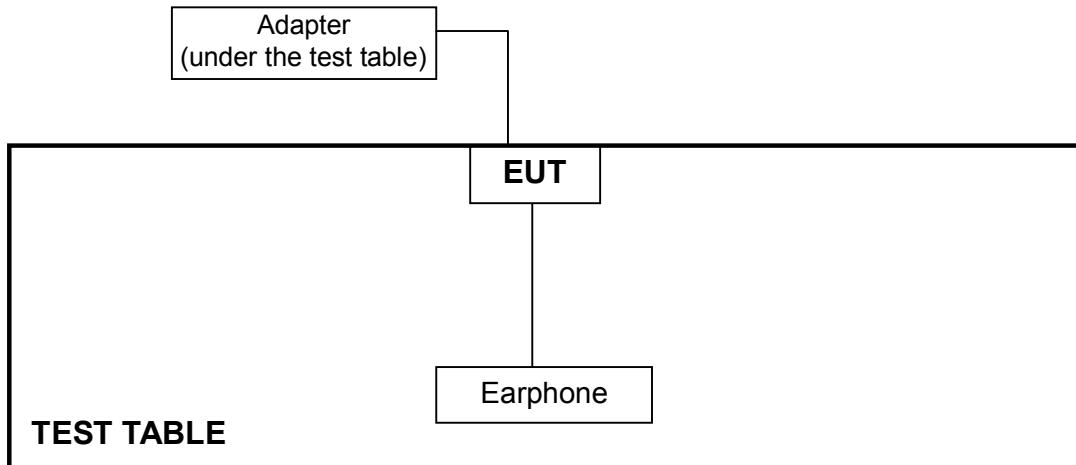
**For Transmitter Radiated Emissions test (30MHz ~ 1GHz) (Test Mode 2):**
