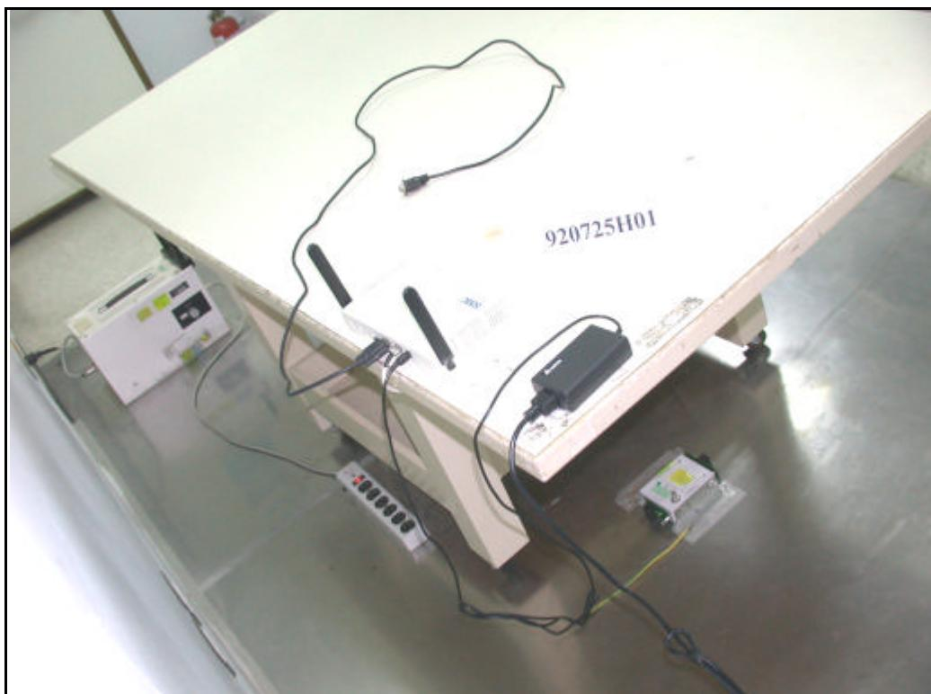
**CONDUCTED EMISSION TEST (With POE)**
