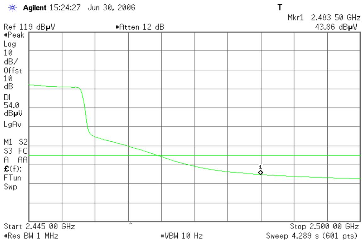
**Band Edges (IEEE 802.11g Turbo Mode / CH Mid)****Detector mode: Peak****Polarity: Vertical**
