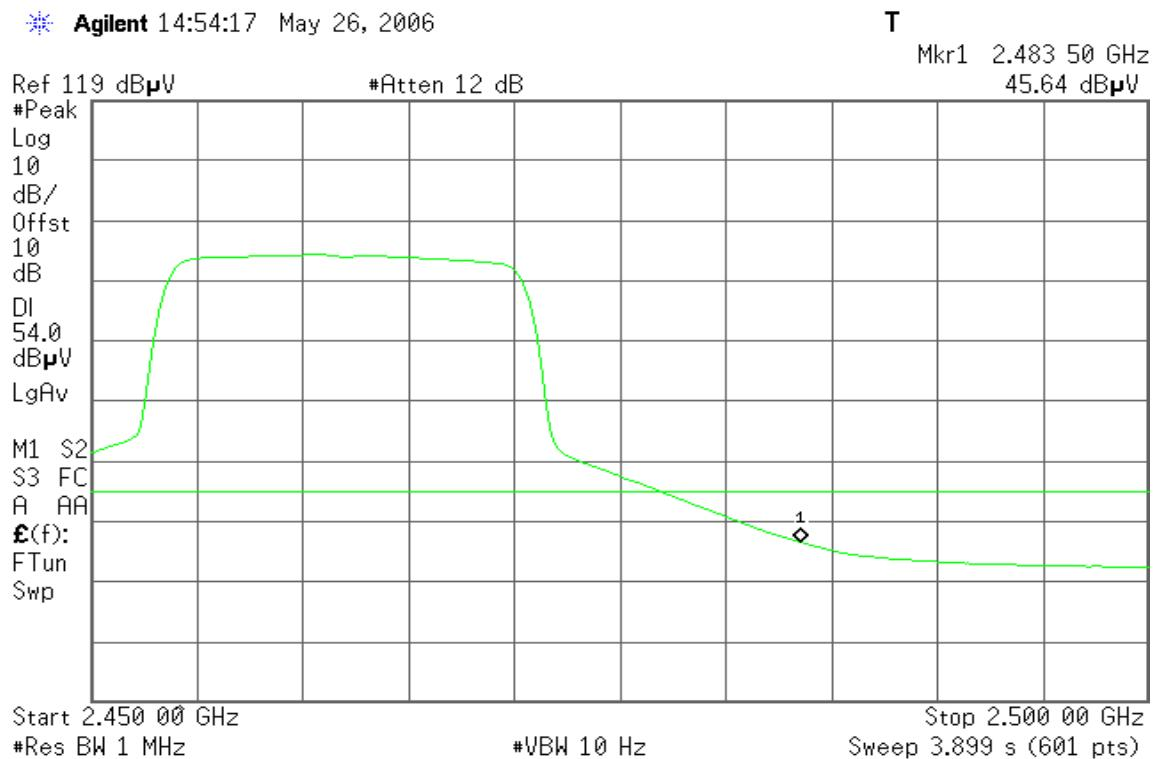
**Band Edges (IEEE 802.11g Turbo Mode / CH Mid)****Detector mode: Peak****Polarity: Vertical**
