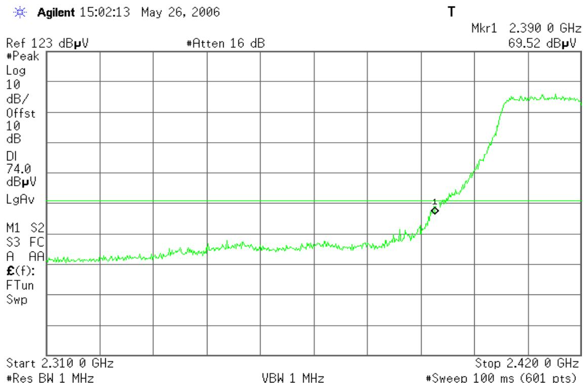
**Detector mode: Average****Polarity: Vertical**
