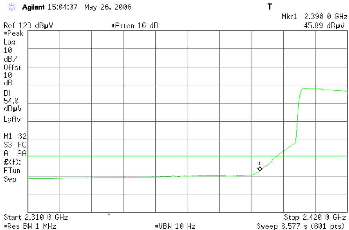
**Band Edges (IEEE 802.11g Base Mode / CH High)****Detector mode: Peak****Polarity: Vertical**
