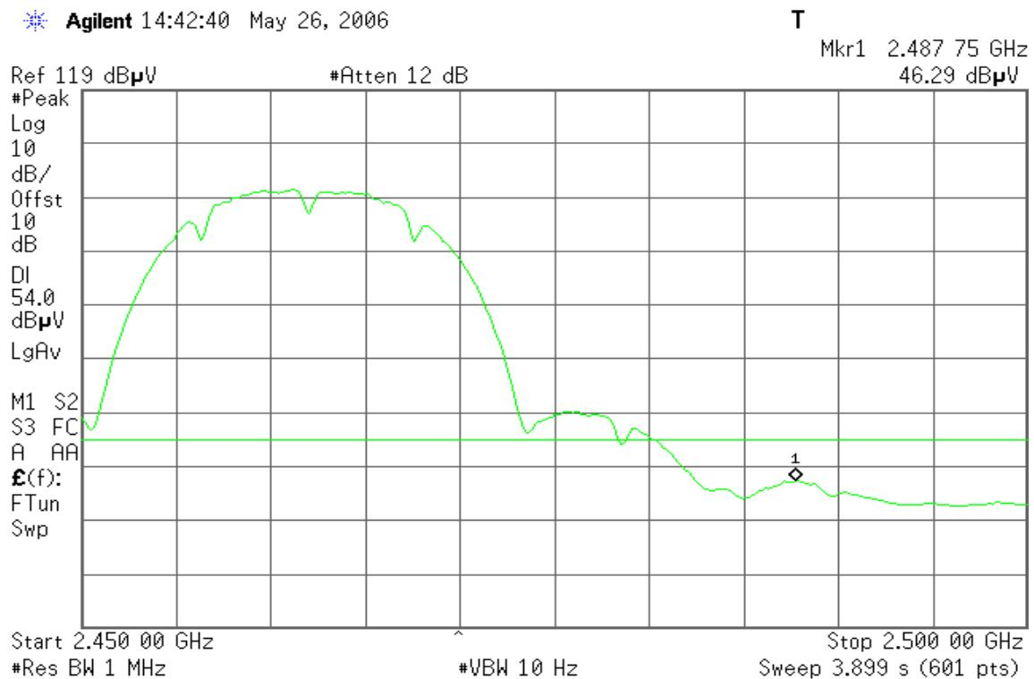
**Band Edges (IEEE 802.11g Base Mode / CH Low)****Detector mode: Peak****Polarity: Vertical**
