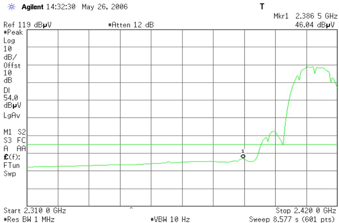
**Band Edges (IEEE 802.11b Base Mode / CH High)****Detector mode: Peak****Polarity: Vertical**
