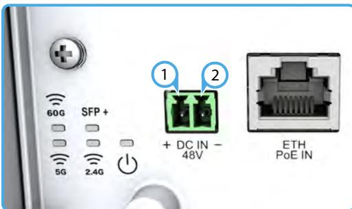
**Warning:** Before wiring the DC block or connecting power to the device, ensure that power to the feed lines is turned off at the supply circuit breaker or disconnected from the power bus.
