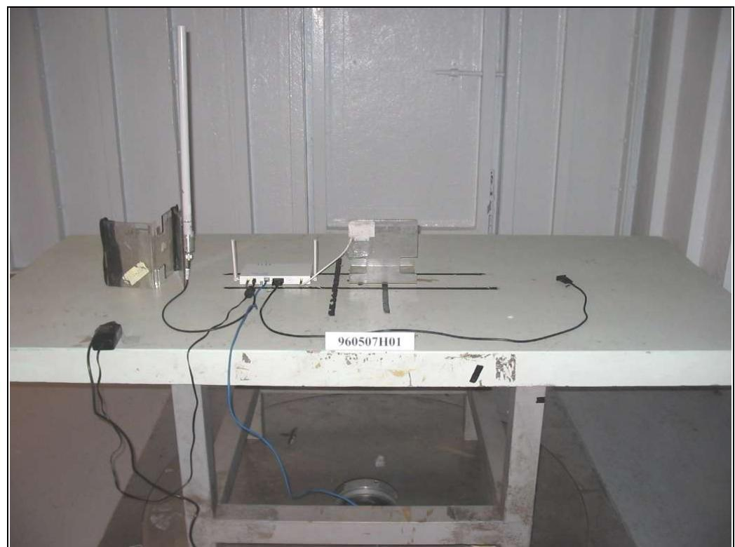
RADIATED EMISSION TEST (2.4GHz Antenna: MP24013XFPT)
