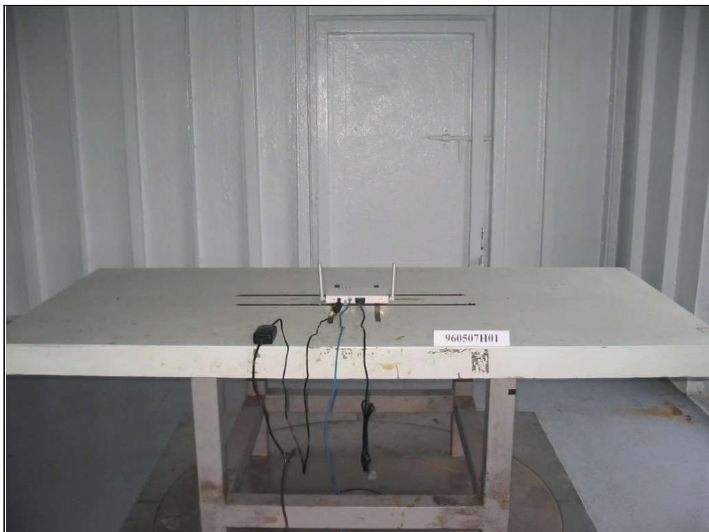
RADIATED EMISSION TEST (5GHz Antenna: MMO24580608)
