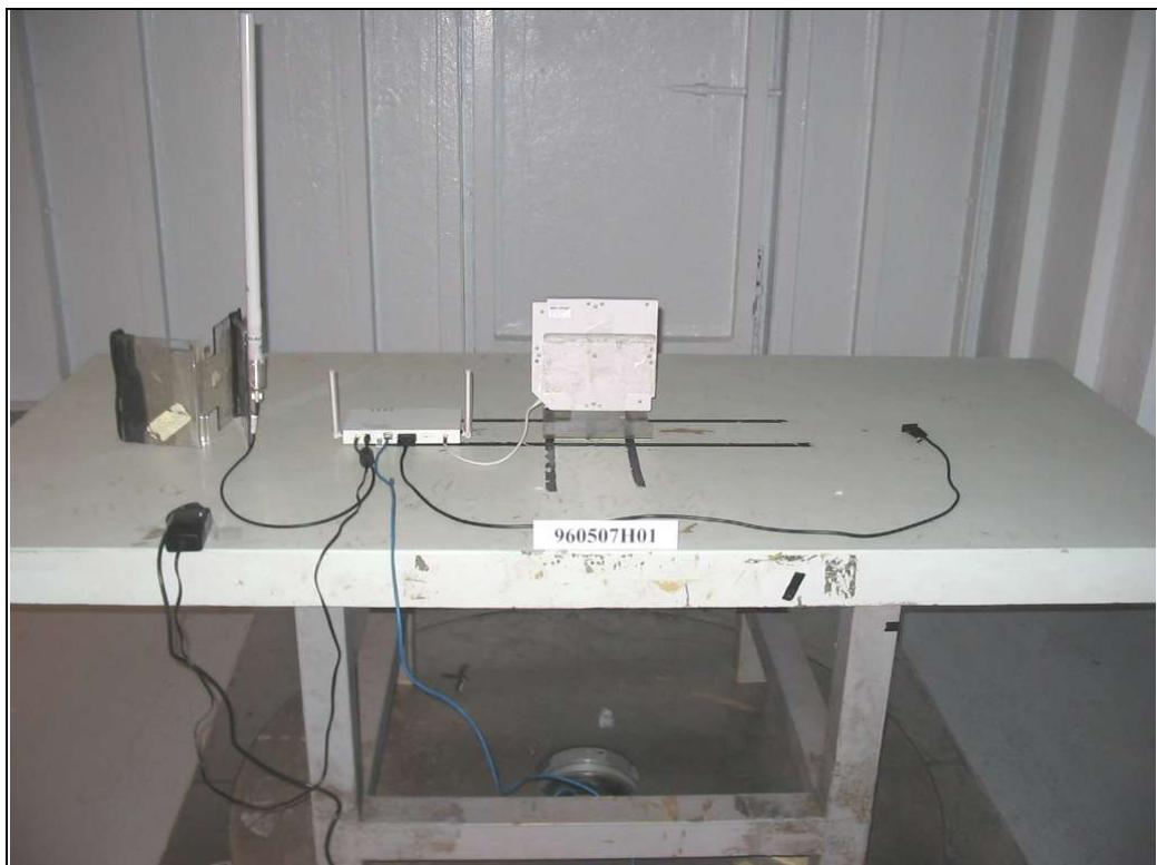
RADIATED EMISSION TEST (2.4GHz Antenna: MMO24580608)
