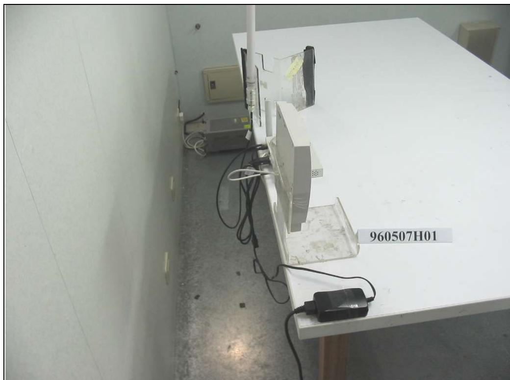
CONDUCTED EMISSION TEST (with POE)
