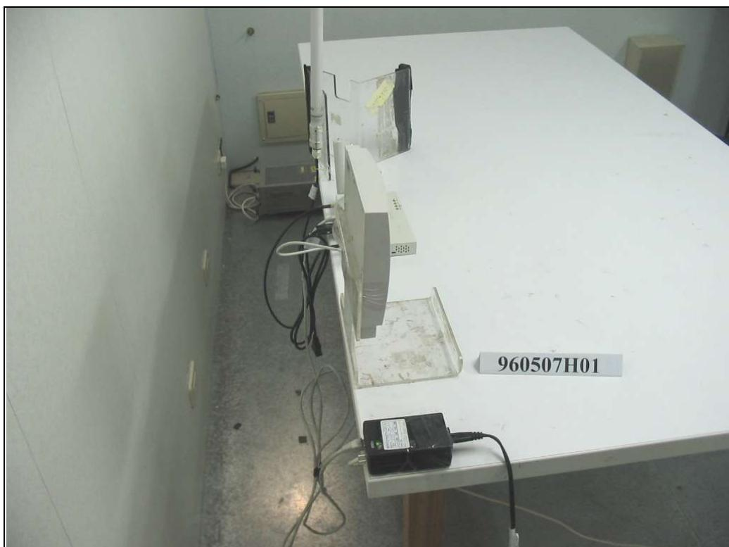
RADIATED EMISSION TEST (2.4GHz Antenna: MHA2400PT)
