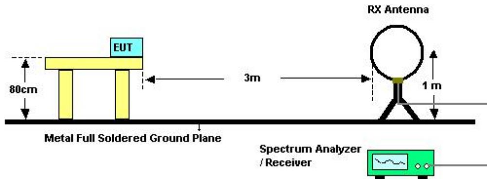
For Radiated Emissions: 30MHz~1GHz
