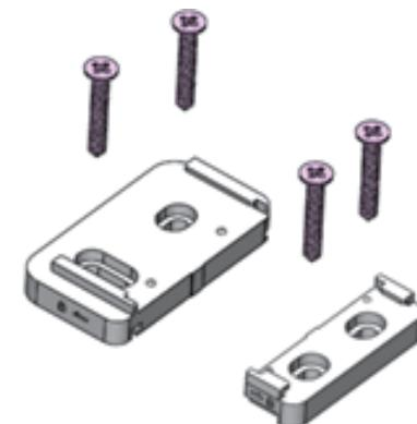
1. Use the supplied wall anchors and screw set to secure the mounting bracket / shim to the wall, door or window frame.
