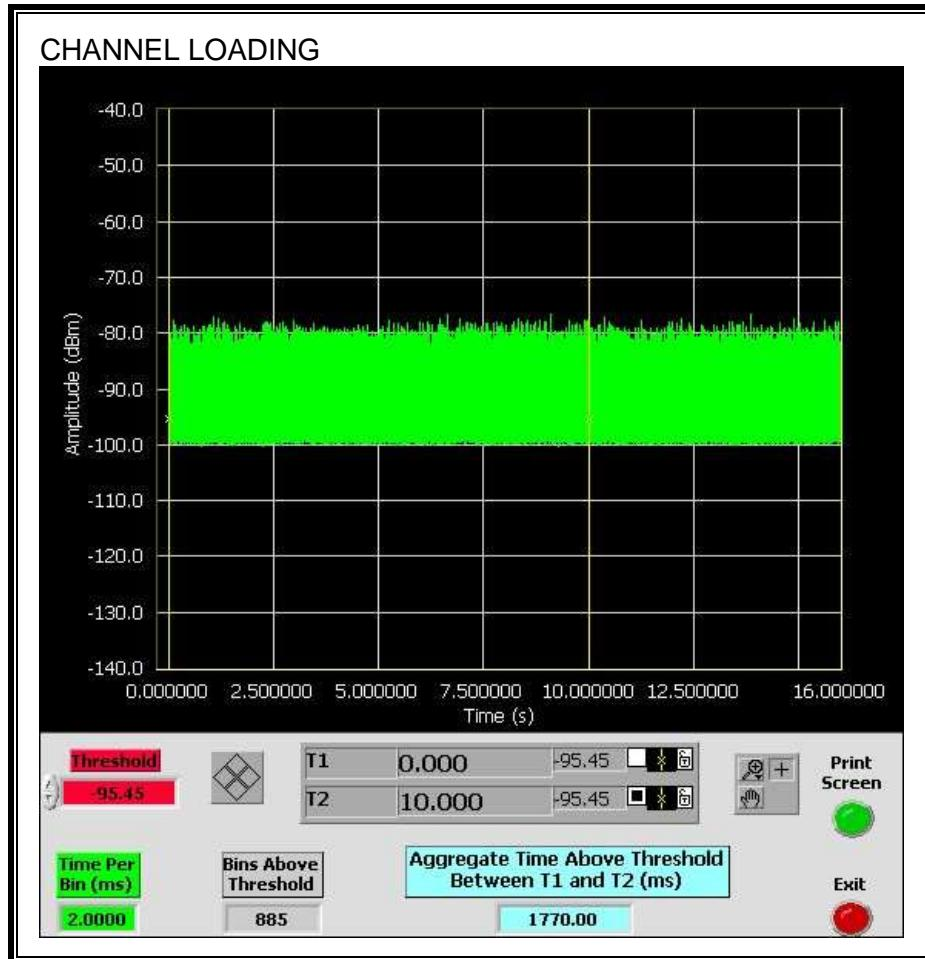
The level of traffic loading on the channel by the EUT is 17.7%
