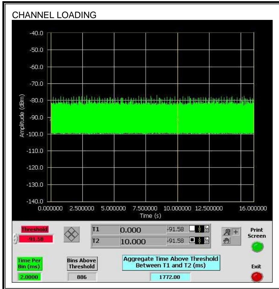
The level of traffic loading on the channel by the EUT is 17.72%
