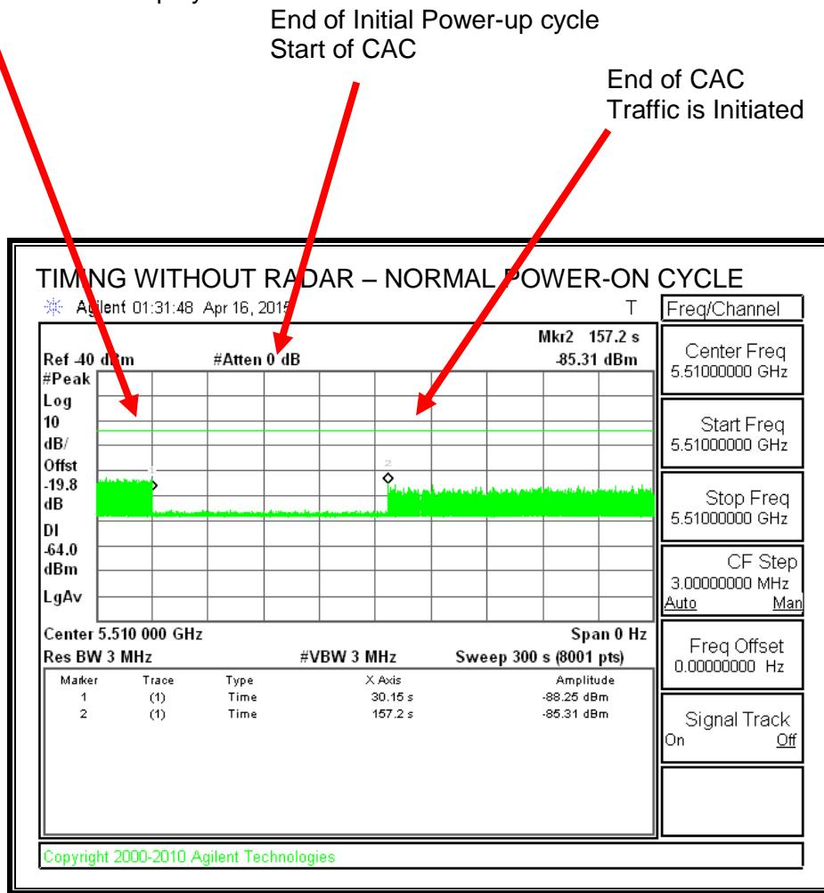
Transmissions begin on channel after completion of the initial power-up cycle and the CAC.
