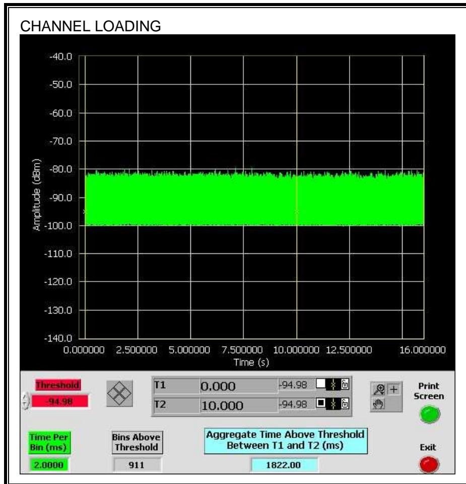
The level of traffic loading on the channel by the EUT is 18.22%
