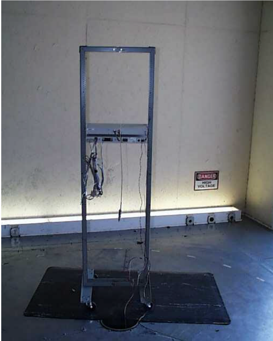
Figure 4: Worst Case Radiated Emissions Setup – Rear View
